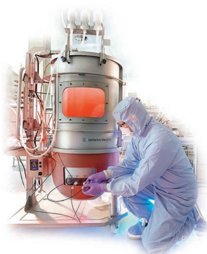
Figure 27.14 A small-scale bioreactor used in vaccine production. Such elaborate systems require the highest levels of sterility and clean techniques. © Photo courtesy of Sartorius Stedim Biotech
