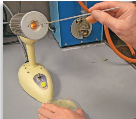
Dry heat incineration. Infrared incinerator with shield to prevent spattering of microbial samples during flaming. © Kathy Park Talaro
