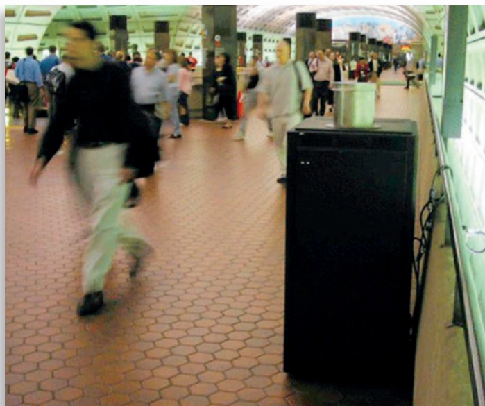
A BioWatch air sampler in the Washington, D.C. subway Courtesy of Lawrence Livermore National Laboratory
