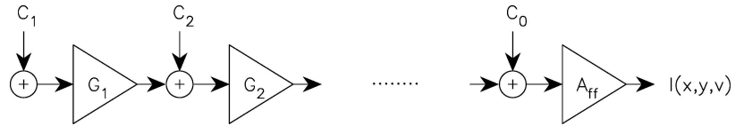
Figure 3. Cascaded amplifiers model. The gain G_i of each amplifier is given by \exp\{\tau_0 \cdot \exp((v - v_j)^2/2\sigma^2)\} Where \sigma = 10 \text{ km s}^{-1} is the internal velocity dispersion of the clumps and v_j is the projected velocity of each clump constituted by a turbulent and a keplerian component. C_i are the continuum contributions between the clumps and A_{ff} is the free-free absorption attenuation. All the parameters are functions of (x, y) .
