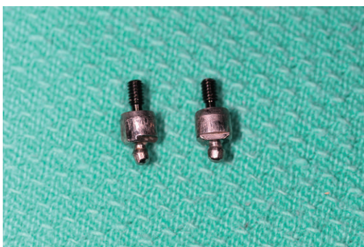
13.11. Mechanical problem: ball abutment wear.
