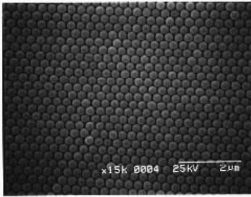
Fig. 1.3. SEM image of a 3D photonic crystal composed of an fcc array of \text{SiO}_2 spheres with a diameter of 300 nm. (After [2])
