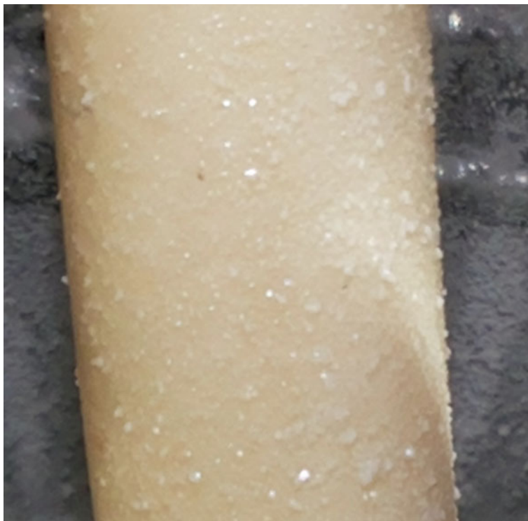
Fig. 10.15 Biocoated surface of silicon rubber
