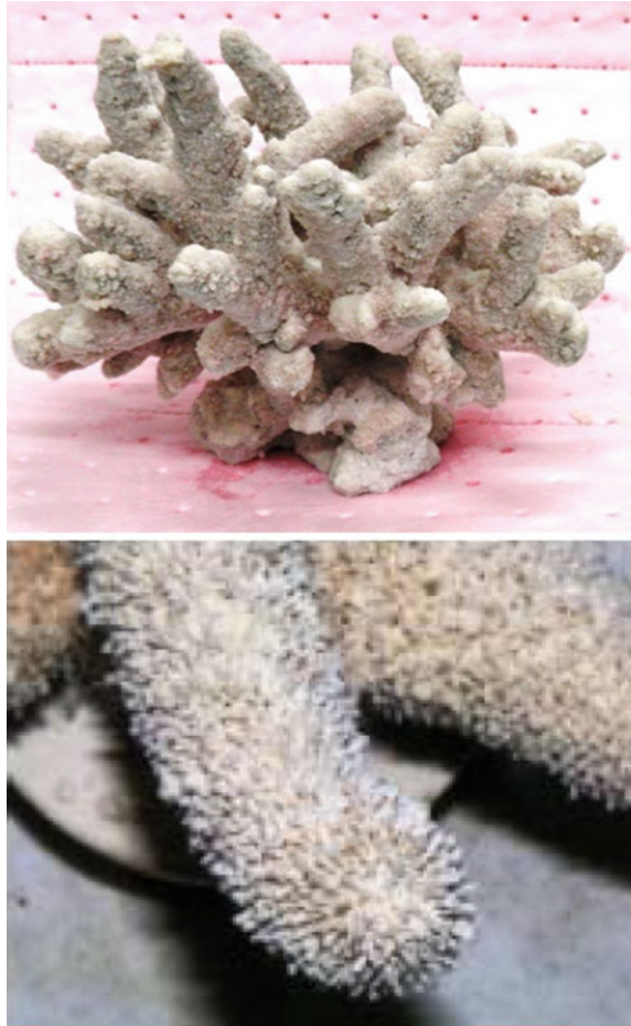
Fig. 10.17 Artificial coral frame coated with calcium carbonate layer for enhanced colonization of corals
