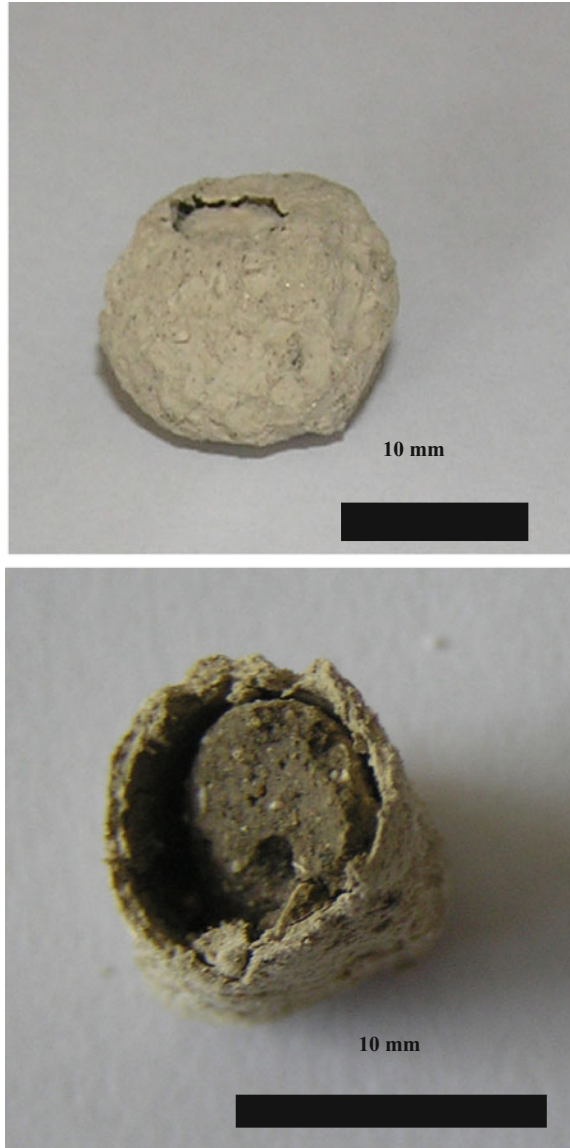
Fig. 10.20 Soft clay aggregates coated with calcite
