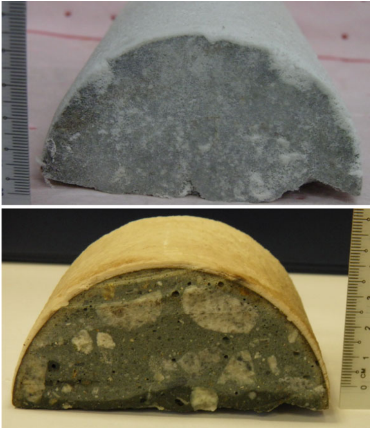
Fig. 10.4 Effect of gravity on MICP on concrete semicylinder before ( upper image ) and after cross section ( bottom image )
