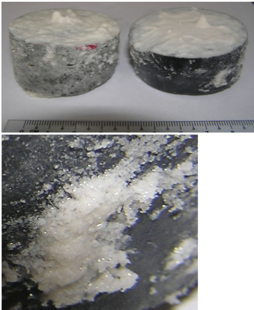
Fig. 10.12 Biocoating of granite and basalt with calcite crystals
