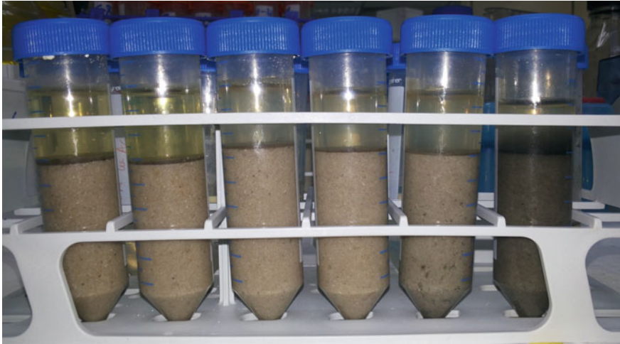
Fig. 7.9 Signs of sulfate-reducing bacteria growth ( black color of CaS and rotten egg smell) appeared after denitrification in the tube containing denitrification medium and 0.05 M of calcium acetate. The tubes contain sand with denitrification medium and following concentration of calcium acetate (from left to right ): 1.0, 0.75 0.5, 0.25, 0.1, and 0.05 M
