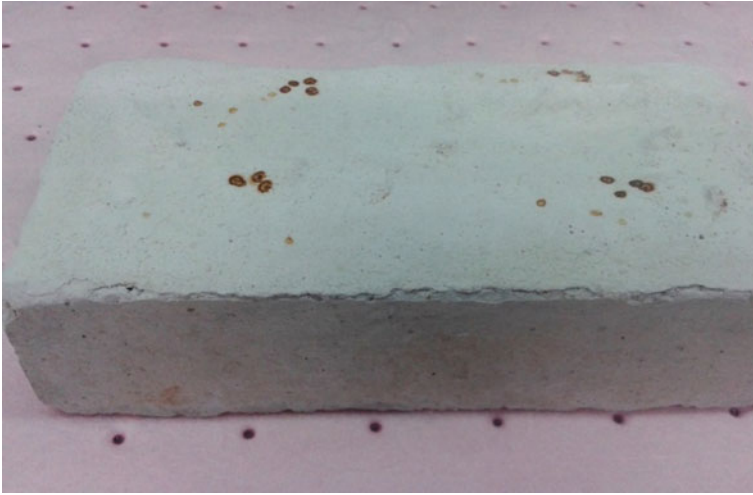
Fig. 10.9 Photo of the coated concrete block after eighth cycles of freezing—heating
