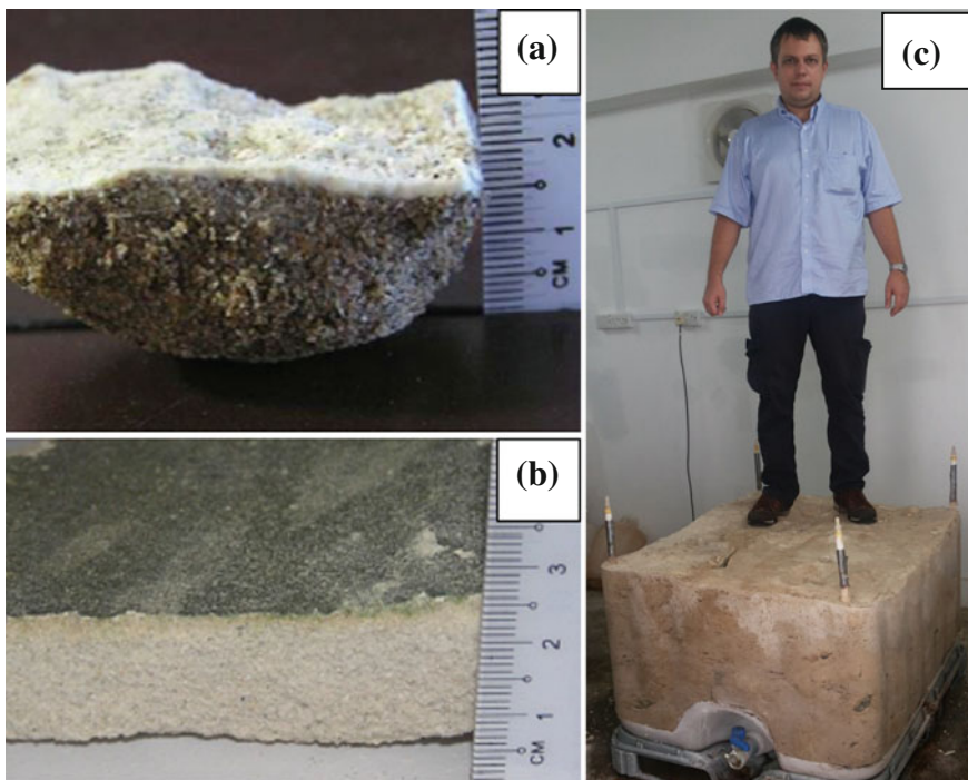
Fig. 7.4 Different spatial types of biocementation: formation of the crust on surface of sand (a), formation of the biocemented layer of the defined thickness (b), bulk biocementation (c)
