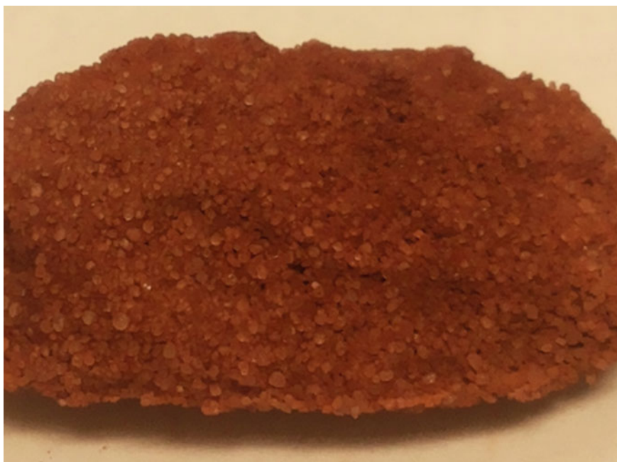
Fig. 8.23 Sand after bioclogging with iron-based biogrowth
