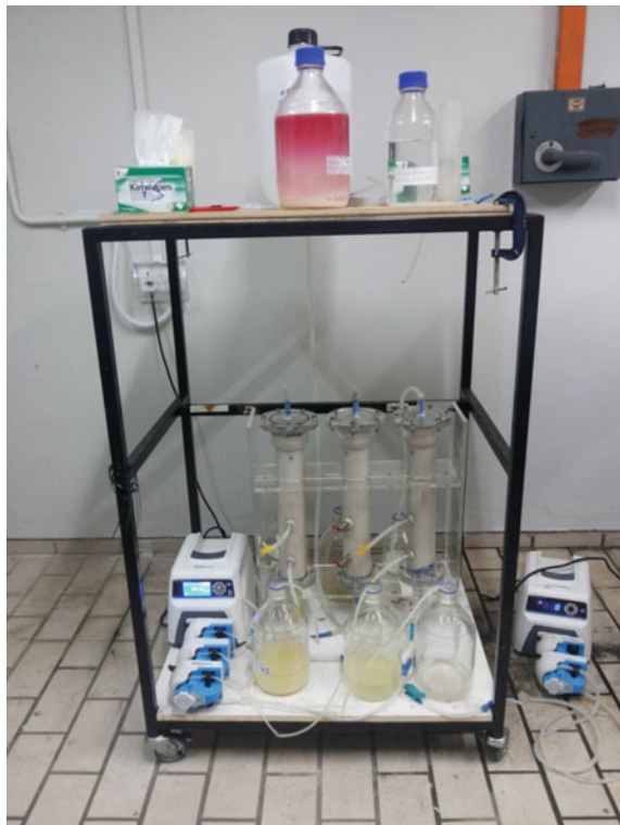
Fig. 8.2 Laboratory facility of three sand columns to study the effect of different biotreatments on hydraulic conductivity of sand. Each acrylic column had an inner diameter 60 mm and height 600 mm. One liter of Ottawa sand was placed into the column. Outlet and inlet of the sand columns were filtered by a layer of 10 mm thick sponge and a layer of 4 mm gravel
