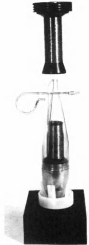
PLATE 8 (top left). "Autosal" laboratory salinometer, water-sample bottles and ampoule of Standard Sea-water.
