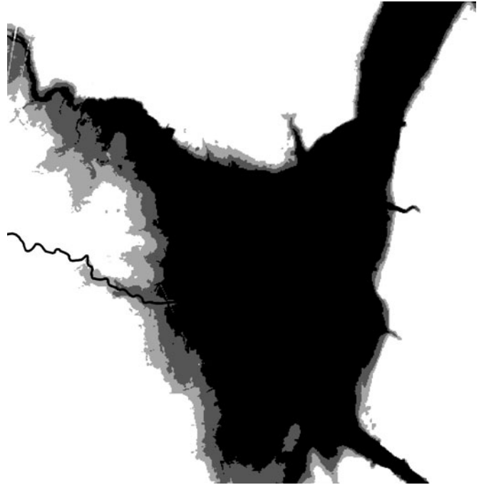
Figure 7.4 Probabilistic floodplain mapping of the 1-in-100 year event (5th, 50th and 95th weighted percentiles; greyscale). This flood inundation map explicitly considers uncertainty in model parameters.
