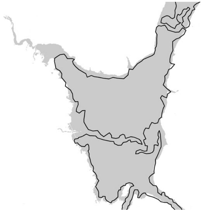
Figure 6.2 Example of simulated flood extent area (in grey) and contour of a SAR-derived flood extent map (black line).
