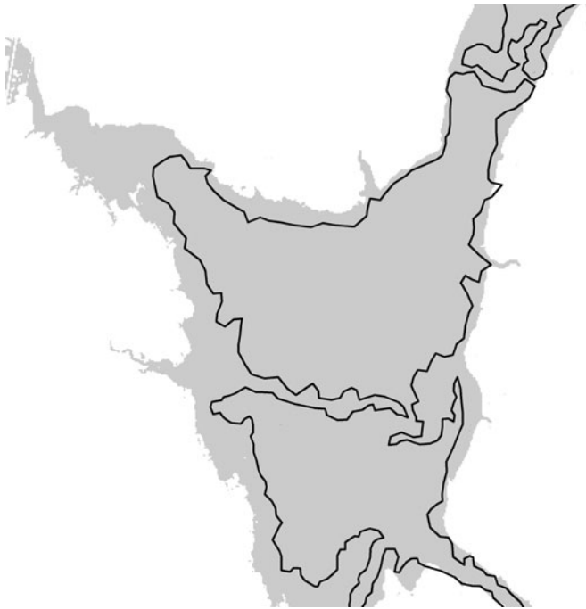
Figure 7.2 Contour of the 2006 flood extent derived from ERS-2 SAR image (black line) and deterministic floodplain mapping of the 1-in-100 year event (grey area).
