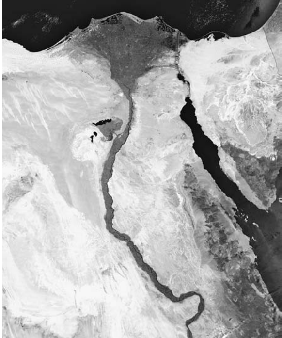
False-color satellite images from the Moderate Resolution Imaging Spectroradiometer (image taken June 3, 2002) showing the Nile River and Delta. The Nile flows from south to north and carries sediment to the Nile Delta, the dark triangular-shaped area at the top of the image. Since many dams, including the Aswân High Dam, were built, the Nile carries less sediment, and the delta is beginning to erode. Also, the fertile Nile Valley is not flooded as often, so the fertilizing silts are no longer deposited on the floodplain. (NASA)
