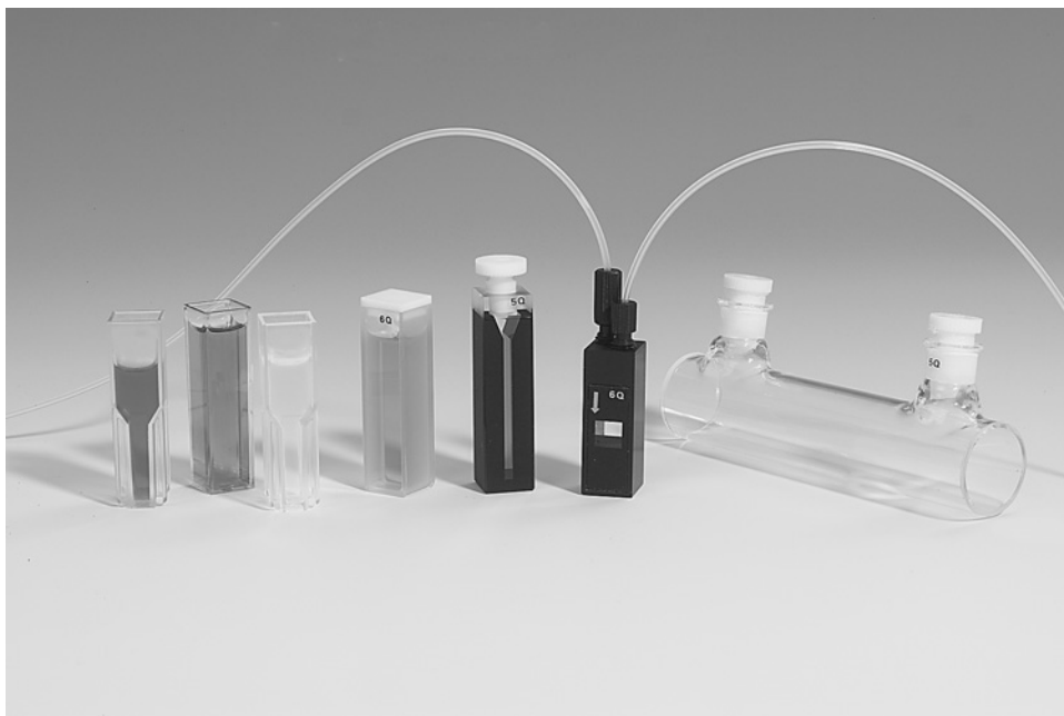
Figure 2.1.2 Collection of commonly used cuvettes (sample cells), differentiated by shape, volume, dimensions, and pathlength. Test tubes and spectropipettors are other types of sample containers.
