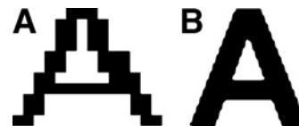
Figure A.3B.1 “Stairstepped” lettering (aliased; A ) and anti-aliased lettering ( B ). Note ghosting of aliased sides of lettering.
