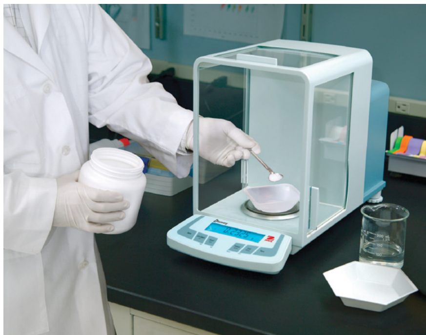
Figure 1.2.5 Weighing boats are available for larger quantities of solid reagents or for liquid reagents.
