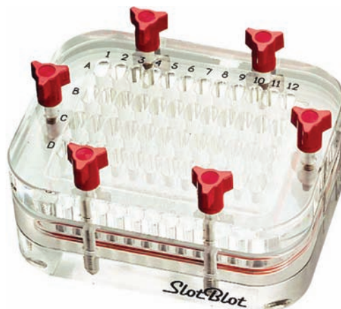
Figure 8.3.3 Slot-blot unit. Through use of a vacuum manifold or by simple hand spotting, up to 96 samples can be applied to a single NC or PVDF membrane for immunoblotting analysis. Although this approach cannot discriminate between the protein of interest and a cross reactive antigen, it is a quick way to perform preliminary characterization and high-volume, routine quantitation of a sample. Figure courtesy of Hoefer, Inc.
