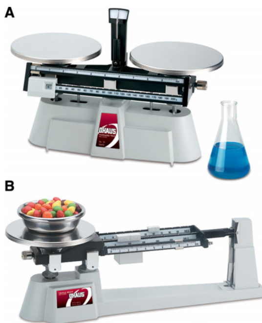
Figure 1.2.1 Examples of mechanical balances. (A) Ohaus Harvard Trip Balance. (B) Ohaus Triple Beam Balance.
