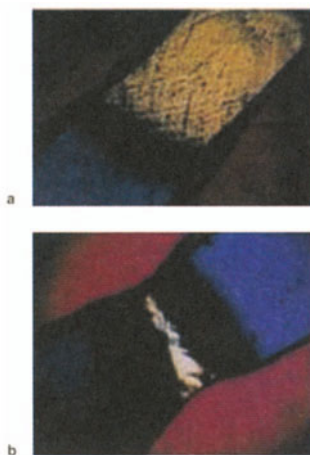
Fig. 15 POM pictures of the neck region of PDES (a) after stabilization (b) when the stress is reduced (after Hedden et al. [82])
