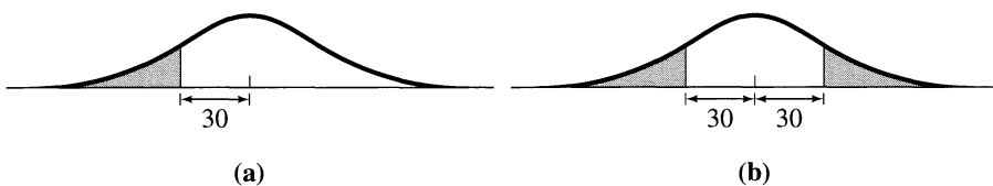
Figure 10.6. (a) The “one-tailed” probability for getting a result 30 or more below the mean. (b) The “two-tailed” probability for getting a result that differs from the mean by 30 or more in either direction. (Not to scale.)
