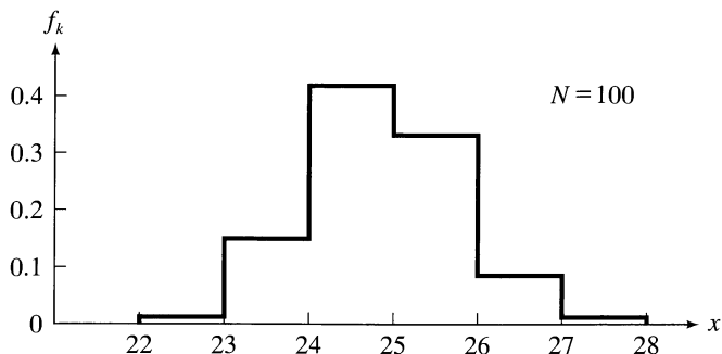
Figure 5.3. Histogram for 100 measurements of the same quantity as in Figure 5.2.
