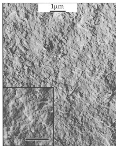
Fig. 39 Fracture surface of a slow-cooled 330 °C/20 min TE-5069 sample. The inset is of a 350 °C, 5 min sample quenched in water
