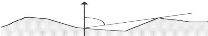
Figure 8: Landscape, consisting of Lambertian surface facets, with horizon at zenith angle \theta_H .
