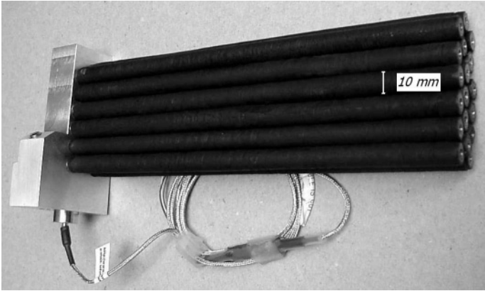
Figure 1. The outward of tube module oxygen storage
