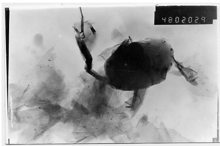
Figure 6. Products of pyrolysis of toluene at temperature 1100 °C, a (X 48 000), b (X48 000).
