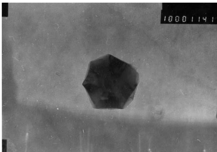
Figure 7. Carbon particle of the polyhedral shape, (X 100 000).
