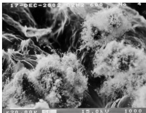
Fig. 3. EG particle covered with carbon nanofibers. Catalyst - nickel
