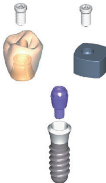
Fig. 58-4 Schematic illustration of the assembly of an orthodontic base on a oral implant designated for prosthetic use after the orthodontic treatment.
