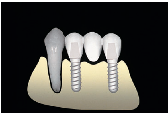
Fig. 54-18 An alternative option would be the replacement of the three missing occlusal units by two implants to support a three-unit suprastructure with a central pontic.
