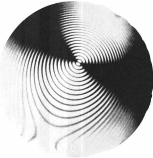
Fig.38. Biaxial, section cut at 80^\circ to optic axis, crystal at 45^\circ position.
