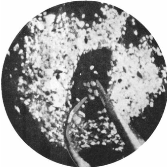
Fig.23. Dielectric separation. The grains attracted to the field between the needle points have dielectric constants greater than 36. The others have smaller dielectric constants and are repelled from the field; \times 70 .
