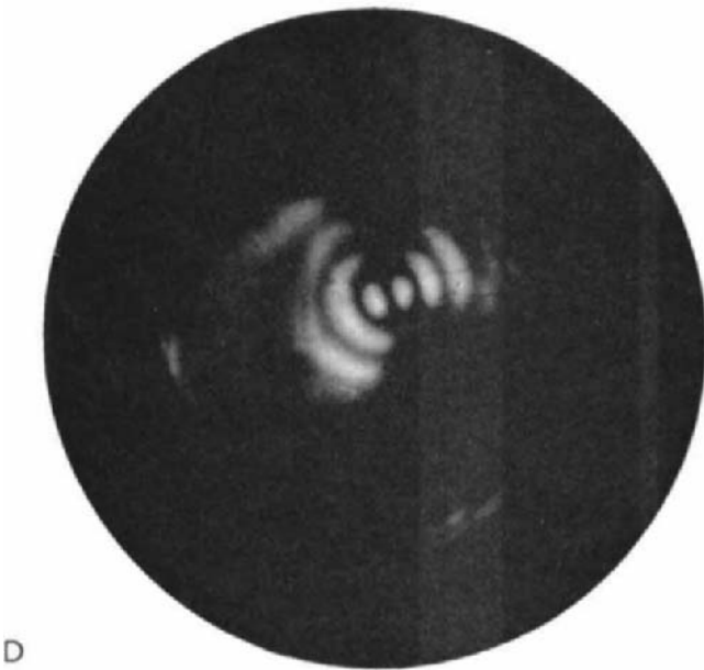
Fig.39. Interference figures photographed with an ordinary petrographic microscope. The visual figures are somewhat better than the photographs portray.
