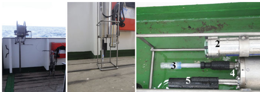
Fig. 9.6 Winch and CTD probe ( left ) and sensing elements ( middle and right ). Number through images: (1) data transfer and power supply cable and connection and rope of winch, (2) oxygen sensor, (3) temperature probe, (4) pressure sensor, (5) conductivity cell
