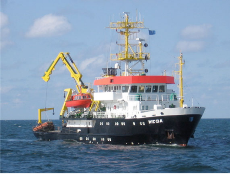
Fig. 9.1 VWFS WEGA, sounding, wreck searching, and research vessel of the BSH. Photo by BSH
