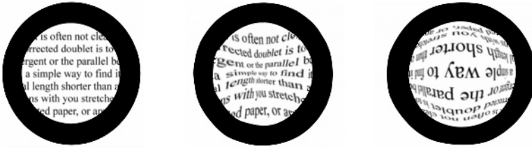
Fig. 7.6 Checking an achromatic doublet corrected for infinite conjugate ratio. If the convergent-beam side is directed to the paper the image remains undistorted when the paper comes close to the focus ( left ). Otherwise the image is distorted ( middle and right )
