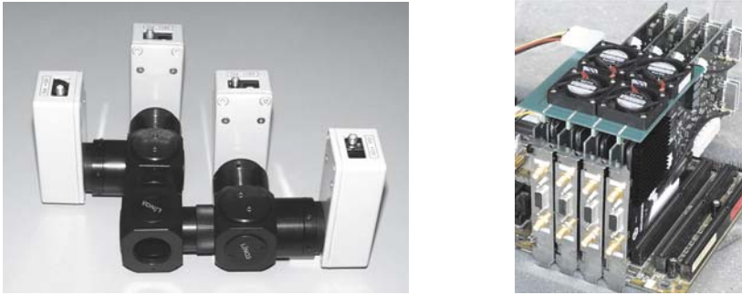
Fig. 5.83 Four-PMT detector assembly ( left ) and four-channel TCSPC imaging system ( right , on a Pentium motherboard)
