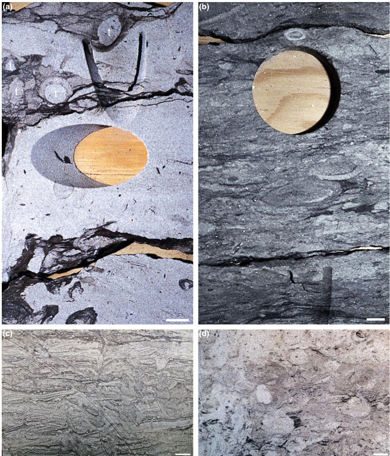
Fig. 5.107 Phycosiphon trochoides in sectioned core. Scale bars = 1 cm. a Heterolithic (silty) sandstone with moderate bioturbation and few burrows in cross section in the upper part ( t ). Middle Jurassic (Bajocian) Ile Formation (shallow marine, prodelta), Norwegian Sea (well 6406/8-1, ca. 4388 m). b Highly bioturbated silty sandstone with oblique burrow sections in the middle. Middle Jurassic (Bajocian) Ile Formation (shallow marine, lower shoreface), Norwegian Sea (well 6406/8-1, ca. 4479 m). c Heterolithic and ripple-laminated sandstone
