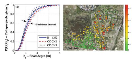
**Fig. 3.15** (a) The fragility curves for the CO limit state for the class of informal building made up of cement-stabilised bricks in Suna neighbourhood (based on 20 simulations); (b) The household risk map: number of people affected (Collapse limit state only) ((Jalayer et al. 2013b) © 2013 Taylor and Francis Group, London UK, used with permission)
