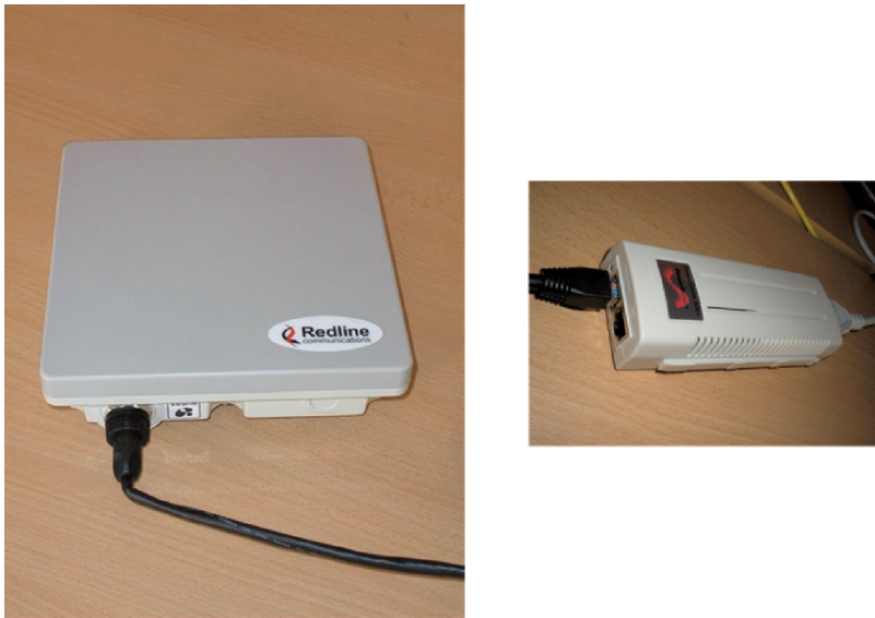
Fig. 7.21. Subscriber station RedMAX SU-O and its power module (PoE)
