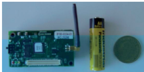
Fig. 7.3. Crossbow Mica-Z mote (W 58 × L 32 × D 7 mm) 6
