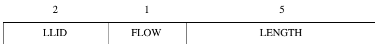
Fig. 3.12. Header of an ACL data packet when transmitted on a single slot
