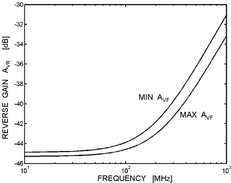
Figure 3.11: Simulated reverse gain  $A_{VR}=20\log_{10}(V_{IN}/V_{OUT})$  versus frequency.
