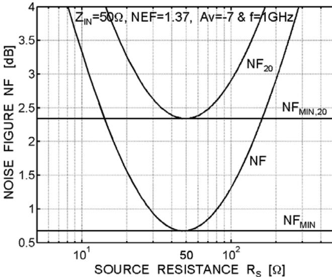
**Figure 4.31:** Simulated NF ( $NF_{20}$ ) and  $NF_{MIN}$  ( $NF_{MIN,20}$ ) versus  $R_S$  for the LNA in figure 4.20c (MOS model 9) for a noiseless (noisy) amplifier “Av”. The matching-stage provides  $R_{IN} \approx 50\Omega$  for  $V_{GS} - V_{T0} \approx 250mV$ .  $R = 300\Omega$  renders a voltage gain ( $=V_V/V_X$ ) of 12.8dB for the matching stage.
