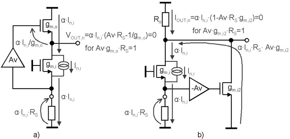
Figure 4.13: Improved noise-cancelling LNAs (biasing not shown).
