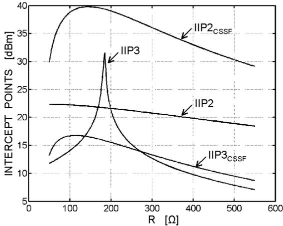
**Figure 5.18:** Simulated 2<sup>nd</sup> and 3<sup>rd</sup> order input-referred intercept points versus  $R$  ( $f_1=10\text{MHz}$ ,  $f_2=12\text{MHz}$ ) for  $\epsilon=0$  and  $C_1=C_2=\text{large}$ .
