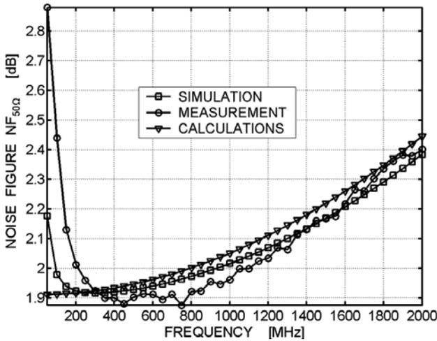
Figure 6.7: Measured and simulated NF versus frequency.
