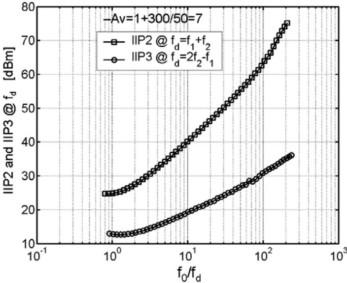
Figure 4.44: Simulated IIP2 and IIP3 versus  $f_0/f_d$ .
