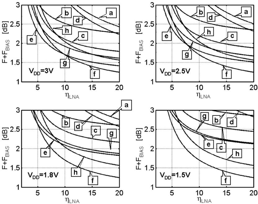
**Figure 4.26:**  $F + F_{\text{BIAS}}$  versus  $\eta_{\text{LNA}}$  for different values of supply voltage  $V_{\text{DD}}$  ( $|A_{\text{VF}}| = 10$ ,  $\text{NEF} = 1.5$ ,  $V_{\text{gs}1} - V_{\text{T}0} = 0.2\text{V}$ ,  $\theta = 0.8 \text{ 1/V}$  and  $\delta = 0.3$  have been assumed).
