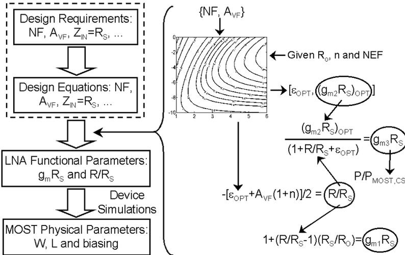
**Figure 5.12:** Description of the LNA design procedure.
