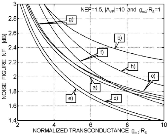
**Figure 4.22:**  $NF$  versus  $g_{m2}R_S$  for  $Z_{IN}=R_S$  and constant  $A_{VF}$ .
