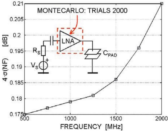
**Figure 5.22:** Montecarlo simulations of process-spread,  $4\text{-}\sigma(\text{NF})$ , versus frequency for  $\epsilon=\epsilon_{OPT}=-4$ .
