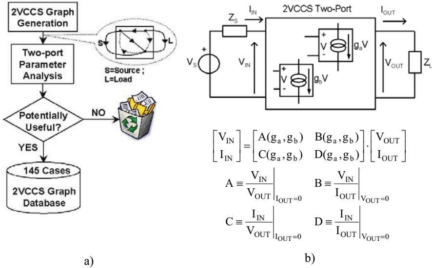
**Figure 2.2:** a) Flow chart describing the steps leading to the generation of the 2VCCS database b) A 2VCCS two-port circuit described by  $\{A, B, C, D\}$  parameters. The latter are a function of the transconductances  $g_a$  and  $g_b$  of the 2 VCCSs (i.e. VCCS<sub>a</sub> and VCCS<sub>b</sub>).
