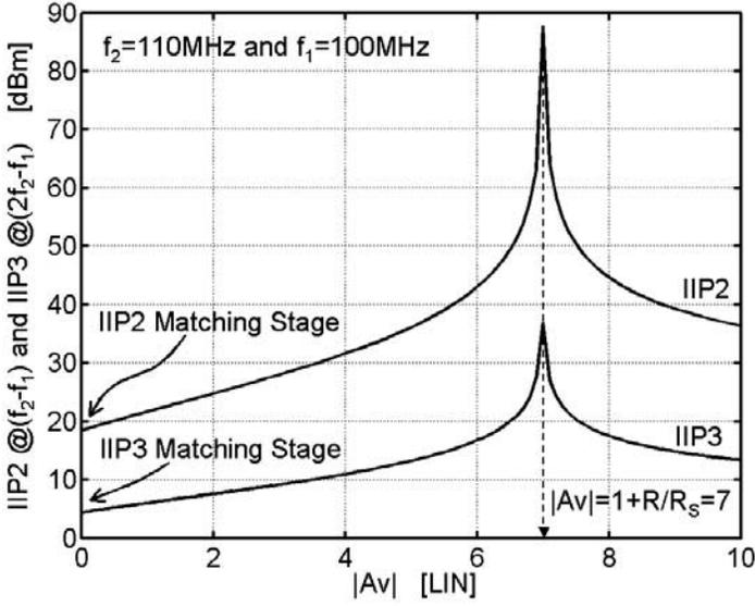
**Figure 4.34:** Simulated IIP2 and IIP3 versus  $|Av|$  for the amplifier in figure 4.32 (MOS model 9). The matching-stage provides  $R_{IN} \approx R_S = 50\Omega$  for  $V_{GS} - V_{T0} \approx 250\text{mV}$  while  $R = 300\Omega$  renders a gain ( $V_Y/V_X$ ) of 12.8dB for the matching stage.
