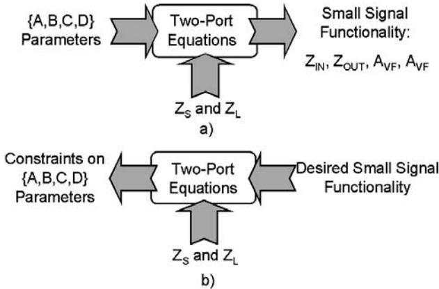
**Figure 2.4:** a)  $\{A, B, C, D\}$  parameters plus  $Z_S$  and  $Z_L$  determine the two-port small-signal functionality. b) Graphs of 2VCCS wideband amplifiers are selected using the reverse reasoning: the desired amplifier functionality is translated into constraints on the  $\{A, B, C, D\}$  parameters upon assigned  $Z_S$  and  $Z_L$ . These constraints are the criteria to select useful graphs within the 2VCCS database.
