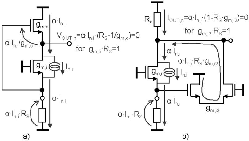
**Figure 4.11:** Wide-band noise-cancelling LNAs (biasing not shown): cancelling of the matching device output noise is indicated.
