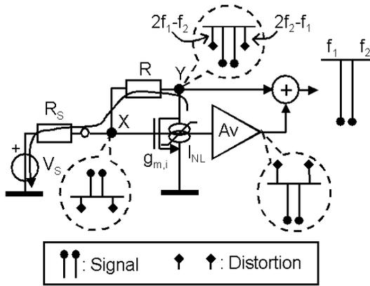
**Figure 4.33:** Cancellation of 3<sup>rd</sup> order intermodulation distortion terms sketched in the frequency domain.
