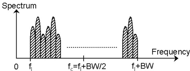
**Figure 1.2:** A wide-band signal spectrum spanning a bandwidth from  $f_1$  to  $f_1+BW$  with centre frequency,  $f_1+BW/2$ , such that the ratio  $BW/(f_1+BW/2)$  can be as large as 2 (i.e. for  $BW/2 \gg f_1$ ).
