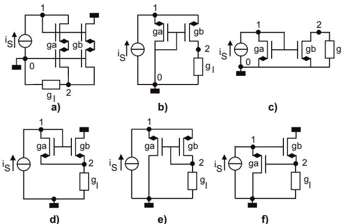
**Figure 6:** Current amplifier approximations derived from the BD graphs (a, b and c) and ABD (d, e, f) graphs with non-unity  $D$ . The current gain of the circuits is either higher than 1 (a, d), lower than 1 (b, e), or arbitrary (c,f).
