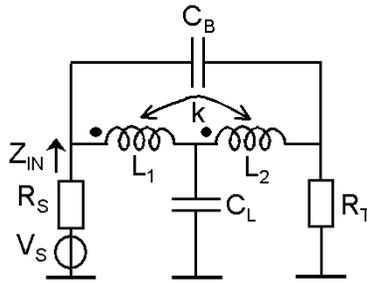
Figure 4.46: Bridged T-coil network.
