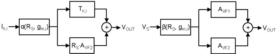
**Figure 4.15:** Block diagram of the matching device noise and input signal transfer.
