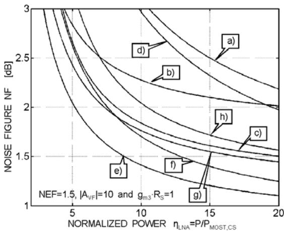
**Figure 4.23:** NF versus  $\eta_{LNA}$  for  $Z_{IN}=R_S$  and constant  $A_{VF}$  ( $\delta=0.3$ ).
