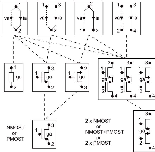
**Figure 4:** The interconnections between the v- and i-branches, and the relative orientation of the branches determines the possibilities to implement a VCCS. Dashed lines show alternative implementations. The double arrow MOST symbol refers to either NMOST or PMOST.
