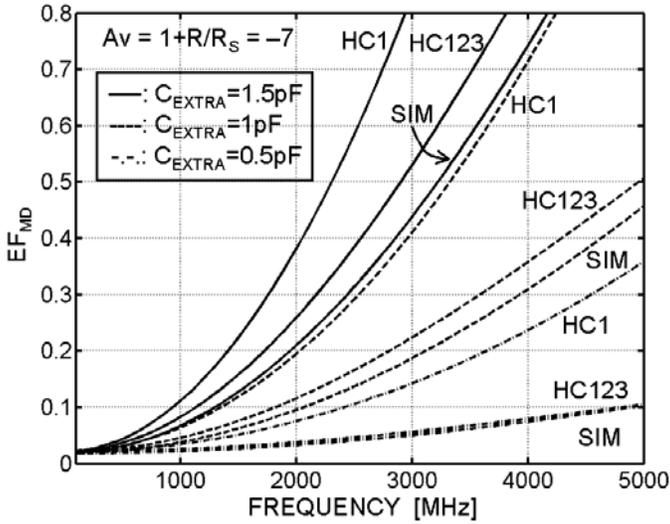
**Figure 4.41:** Simulated (SIM) and hand-calculated (HC)  $EF_{MD}$  versus frequency for different values of  $C_{EXTRA}$  (HC1 refers to the case when only  $C_1$  is present and HC123 refers to case where  $C_1$ ,  $C_2$  and  $C_3$  are present).  $NEF=1.37$ .
