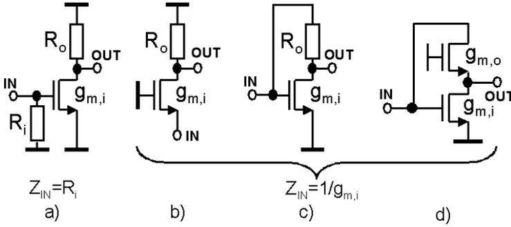
**Figure 4.2:** Elementary wide-band LNAs (biasing not shown): a) CS stage plus resistive termination (CST), b) CG stage, c) CS shunt feedback stage (CSSF) and d) amplifier A1 (“i” and “o” refer to the input and output devices).
