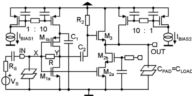
Figure 6.6: Complete schematic of the designed wide-band noise cancelling LNA.
