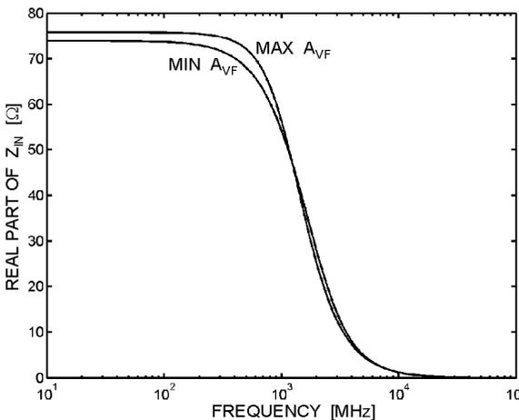
Figure 3.9: Simulated real part of the input impedance versus frequency.
