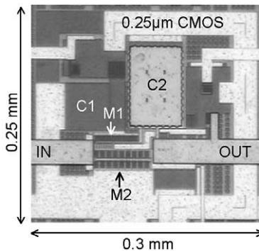
**Figure 5.23:** Die-photo of the wide-band 0.25μm CMOS LNA.
