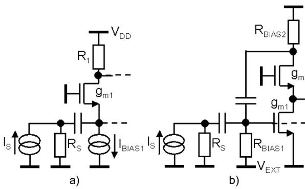
**Figure 1:** Biasing of the matching stage used in the LNAs of figure 4.16.
