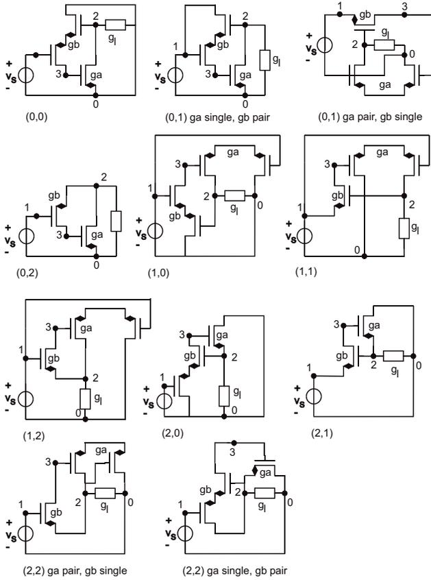
**Figure 8:** Voltage follower circuits derived from the graph in Figure 7 by systematically connecting the  $v_a$ \_ref and  $i_b$ \_ref nodes to all other nodes in the circuits (their node numbers are indicated between brackets).
