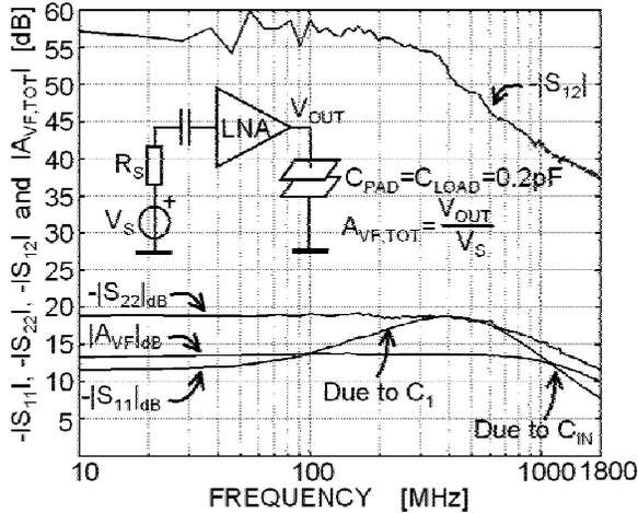
**Figure 5.24:** Measured (on-wafer)  $S_{11}$ ,  $S_{22}$ ,  $S_{12}$  and  $A_{VF,TOT}$  versus frequency.
