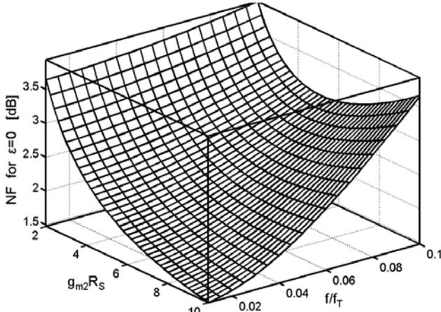
**Figure 5.7:** NF at  $\epsilon=0$  versus  $(g_{m2}R_S, f/f_T)$  for  $A_{VF}=-10$ ,  $n=0.2$ ,  $NEF=1.5$ ,  $R_O=1K\Omega$ ,  $L_{min}=0.25\mu m$ ,  $\alpha_{ov,n}=0.2$ ,  $\alpha_{ov,p}=0.5$ ,  $\alpha_{jn}=0.32$ ,  $\alpha_{jp}=0.28$  and  $\alpha_{np}=2.5$ .
