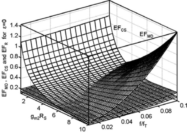
**Figure 5.6:** EF's at  $\epsilon=0$  versus  $(g_{m2}R_S, f/f_T)$  for  $A_{VF}=-10$ ,  $n=0.2$ ,  $NEF=1.5$ ,  $R_O=1K\Omega$ ,  $L_{min}=0.25\mu m$ ,  $\alpha_{ov,n}=0.2$ ,  $\alpha_{ov,p}=0.5$ ,  $\alpha_{jn}=0.32$ ,  $\alpha_{jp}=0.28$  and  $\alpha_{np}=2.5$ .
