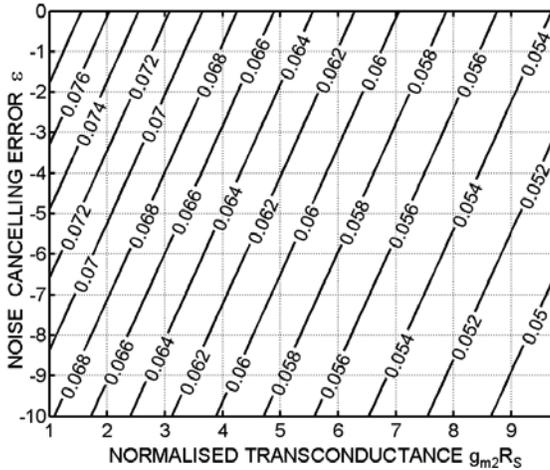
**Figure 5.11:** Contours of  $f_{3dB}/f_T$  versus  $(\epsilon, g_{m2}R_s)$  for  $A_{VF}=-10$ ,  $n=0.2$ ,  $NEF=1.5$ ,  $R_O=1K\Omega$ ,  $L_{min}=0.25\mu m$ ,  $\alpha_{ov,n}=0.2$ ,  $\alpha_{ov,p}=0.5$ ,  $\alpha_{jn}=0.32$ ,  $\alpha_{jp}=0.28$  and  $\alpha_{np}=2.5$ .
