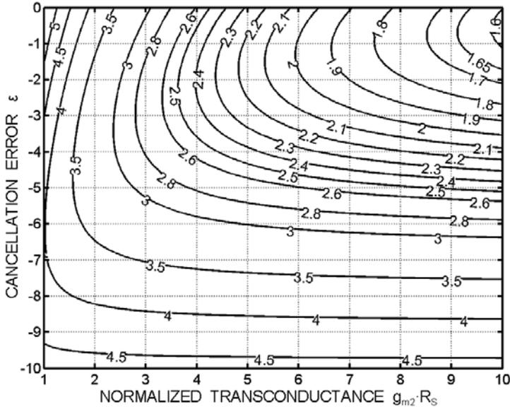
Figure 5.4: Contour lines of the LNA noise figure  $NF(\epsilon, g_{m2}R_S)$  for  $n=0$  and  $R_o=\infty$ .
