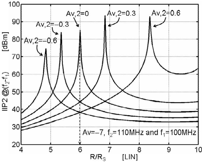
**Figure 4.35:** Simulated IIP2 versus  $R/R_S$  for different values of  $A_{v,2}$  (MOS model 9) for the amplifier in figure 4.33. The matching-stage provides  $R_{IN} \approx R_S = 50\Omega$  for  $V_{GS} - V_{T0} \approx 250\text{mV}$  while  $R = 300\Omega$  renders a voltage gain ( $=V_Y/V_X$ ) of 12.8dB for the matching stage.
