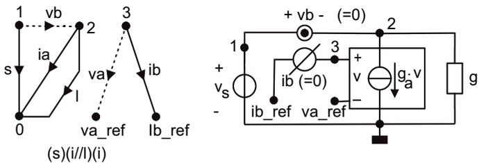
**Figure 7:** The voltage follower graph  $(s)(i//l)(i)$  in which VCCSb acts as a nullor, that forces the load voltage equal to the source voltage.
