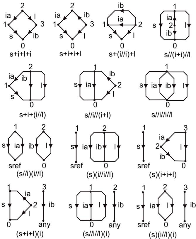
**Figure 3:** The 13 directed labeled Kirchhoff Current Law graphs for two-ports with two VCCSs. By adding  $v_a$ - and  $v_b$ - branches systematically between all possible combinations of nodes, all graphs for two-ports with 2 VCCSs are generated.
