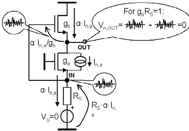
**Figure 3.4:** Cancelling of the output noise voltage due to the matching device noise current,  $I_{n,a}$ .
