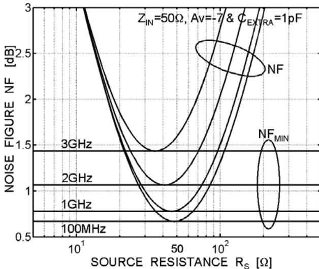
**Figure 4.43:** Simulated NF and  $NF_{MIN}$  of the amplifier in figure 4.38b ( $R_{IN}=50\Omega$  and  $-A_V=1+300/50=7$ ) versus  $R_S$  at different frequencies for  $C_{EXTRA}=1\text{pF}$ .
