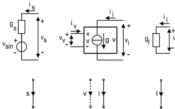
**Figure 1:** Circuit elements and their graph representations: an independent source (s-branch), a VCCS (v- and i-branch) and a load impedance (l-branch).
