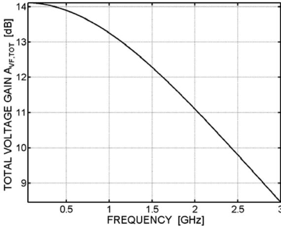
**Figure 5.21:** Total voltage gain  $A_{\text{VF,TOT}}$  versus frequency (50MHz to 3GHz) for  $\epsilon = \epsilon_{\text{OPT}} = -4$ .
