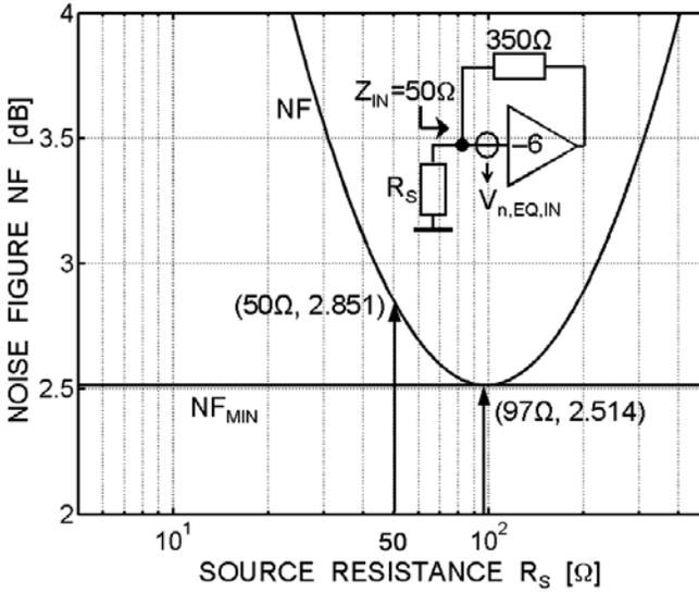
**Figure 4.32:** Simulated NF and  $NF_{MIN}$  versus  $R_S$  of the LNA in figure 4.7-III for a noisy amplifier “Av” with  $R_{n,EQ,IN}=30\Omega$ .
