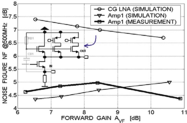
**Figure 6.3:**  $NF_{50}@500\text{MHz}$  versus  $A_{VF}$  for the LNA of figure 6.2 and a CG amplifier derived from it (see text).
