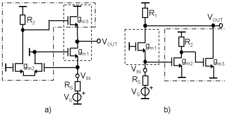
**Figure 4.17:** Two-port model of the amplifiers “a” and “b” in figure 4.16 (biasing not shown).
