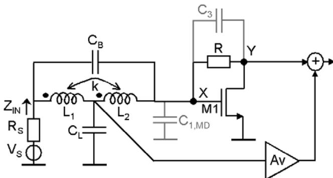
**Figure 4.47:** Frequency compensated noise-cancelling LNA exploiting the bridged T-coil network in figure 4.46.
