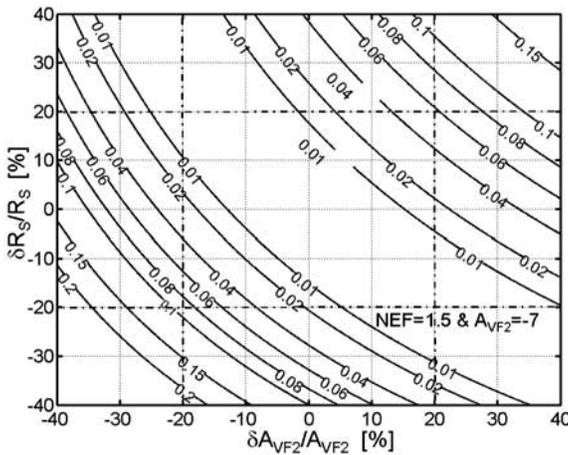
**Figure 4.29:** Contour of  $\delta EF_{MD}$  vs.  $\delta A_{VF2}/A_{VF2}$  and  $\delta R_S/R_S$ .
