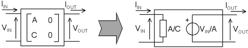
**Figure 2.7:** A two-port circuit with parameters  $\{A, 0, C, 0\}$ .
