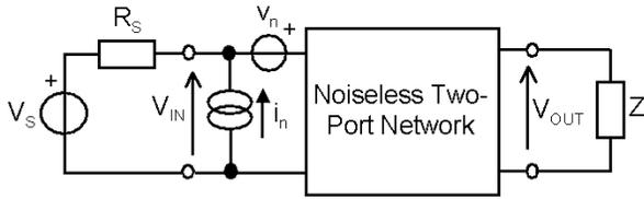
**Figure 1:** Two-port circuit noise model.
