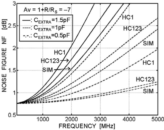
**Figure 4.42:** Simulated (SIM) and hand-calculated (HC)  $EF_{MD}$  versus frequency for different values of  $C_{EXTRA}$  (HC1 refers to the case when only  $C_1$  is present and HC123 refers to case where  $C_1$ ,  $C_2$  and  $C_3$  are present).  $NEF=1.37$
