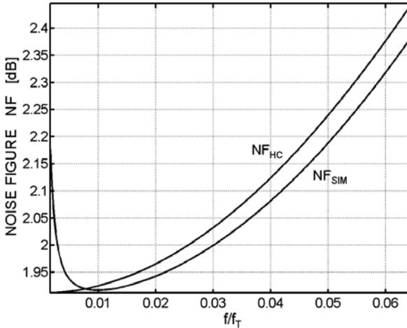
**Figure 5.20:** Simulated  $\text{NF}_{\text{SIM}}$  and calculated  $\text{NF}_{\text{HC}}$  versus  $f/f_T$  ( $f_T = 31\text{GHz} @ V_{GS}\text{-}V_{T0}=250\text{mV}$ ) for  $\epsilon = \epsilon_{\text{OPT}} = -4$ .
