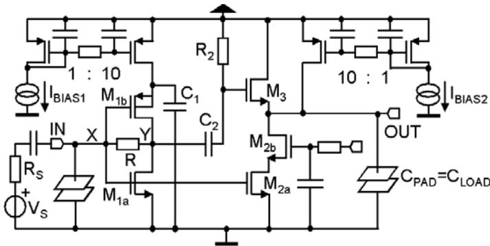
Figure 5.1: Schematic of the selected wide-band LNA circuit.
