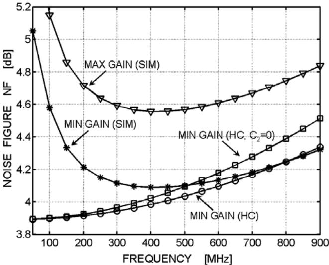
**Figure 3.12:** NF for  $R_S=75\Omega$  versus frequency (HC=Calculations; SIM=Simulations).
