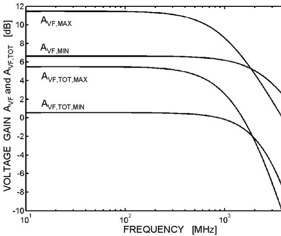
Figure 3.8: Simulated amplifier voltage gains  $A_{VF}$  and  $A_{VF,TOT}$ .
