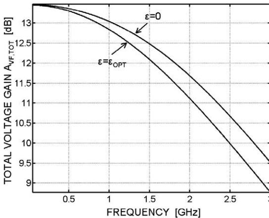
**Figure 5.17:** Total gain,  $A_{VF,TOT}$  versus frequency for  $\epsilon=0$  and  $\epsilon=\epsilon_{OPT}=-4.5$ .
