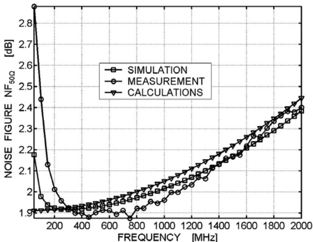
Figure 5.26: Measured, simulated and calculated NF versus frequency.
