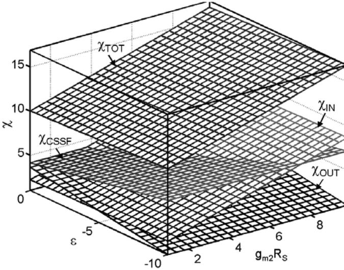
**Figure 5.10:**  $\chi$  versus ( $\epsilon$ ,  $g_{m2}R_S$ ) for  $A_{VF}=-10$ ,  $n=0.2$ ,  $NEF=1.5$ ,  $R_O=1K\Omega$ ,  $L_{min}=0.25\mu m$ ,  $\alpha_{ov,n}=0.2$ ,  $\alpha_{ov,p}=0.5$ ,  $\alpha_{jn}=0.32$ ,  $\alpha_{jp}=0.28$  and  $\alpha_{np}=2.5$ .
