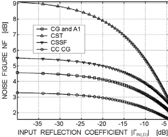
**Figure 4.5:** NF versus  $|\Gamma_{IN(D)}$  for  $|A_{VF,TOT}|=5$  ( $NEF=1.5$ ).
