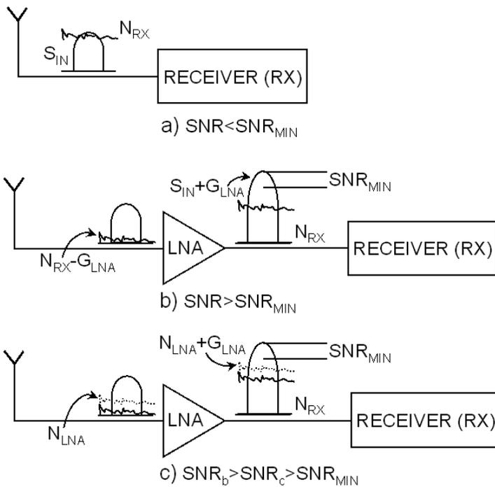
**Figure 1.1:** Placing a Low-Noise Amplifier in front of a receiver to improve its sensitivity: a) w/o LNA, b) w noiseless LNA and c) w LNA noise included. All the quantities are in dB's.
