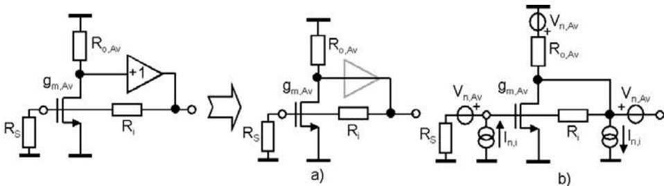
Figure 4.10: Alternative implementations of the feedback LNA in figure 4.8c (biasing not shown).
