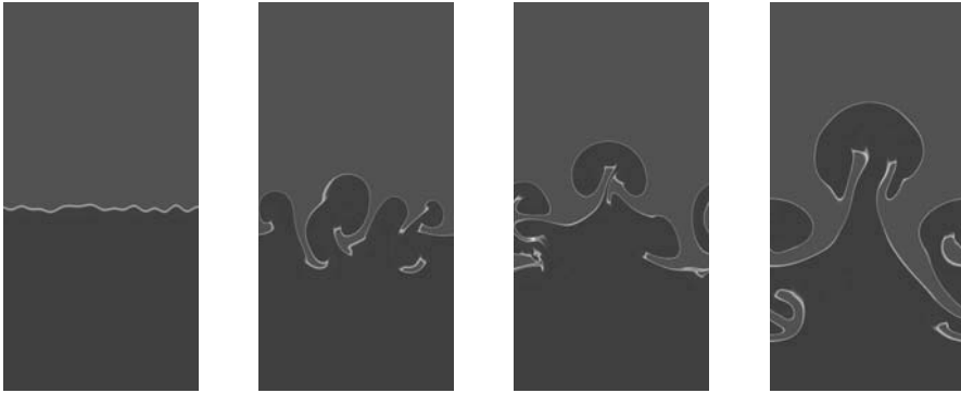
Fig. 5. Time sequence of Rayleigh Taylor unstable nuclear flame at density fuel density 1.5 \times 10^7 g/cc. Times are 0.0, 0.7, 1.1 and 1.4 msec. The image shows carbon mass fraction with red to blue corresponding to high to low values.
