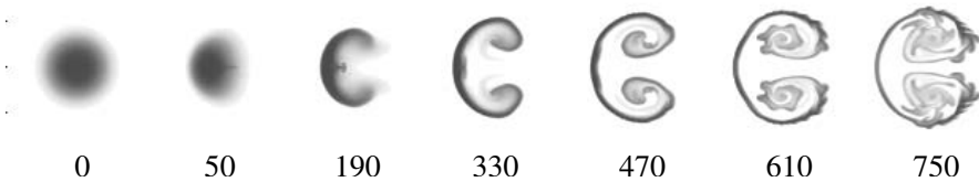
Fig. 2. Evolution of the SF_6 , with time elapsed after shock impact listed in \mu s . The mass fraction of SF_6 is shown, with X_{SF_6}=0.6 and CFL=0.8 .
