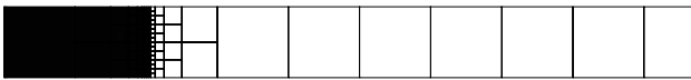
Fig. 5. Half of the domain for the initial condition of a detonation, where the long domain is refined nowhere except at a sharp interface. The domain originally consists of a top-level mesh of 1 \times 20 blocks. This mesh is then refined at an interface. Shown is the meshes 6, zoomed in near the interface. Not shown are 10 coarsest blocks to the right.
