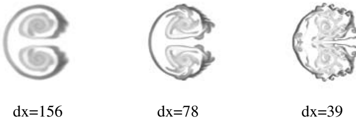
Fig. 4. \text{SF}_6 mass fraction at 750\mu\text{s} with increasing grid resolution, labeled in microns. At the highest level of resolution, the vortex cores appear diffuse.
