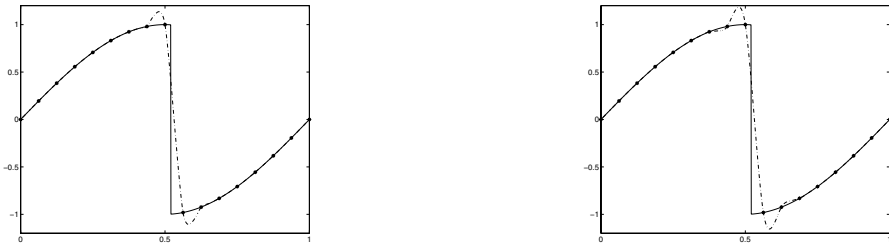
Fig. 2. A piecewise smooth signal (solid line) and its point-values on a uniform grid (dots on solid line). Interpolatory reconstructions (Dotted lines). Left: p = 1, N = 3 . Right p = 2, N = 5 .
