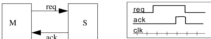
Figure 7-1. Master-Slave Handshake Protocol
