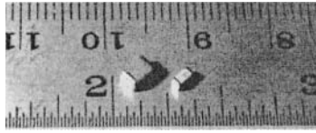
Figure 2-5. SMD digital component sizes
