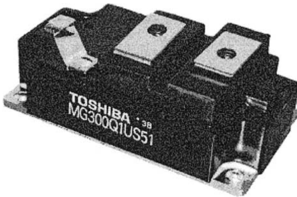
Figure 3-1. A high-power silicon IGBT from Toshiba Semiconductor
