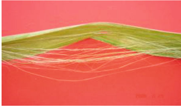
Fig. 2.32 Separating fibres from soft covering material (Courtesy of Dr. Januar Parlaungan Siregar, Universiti Malaysia Pahang)
