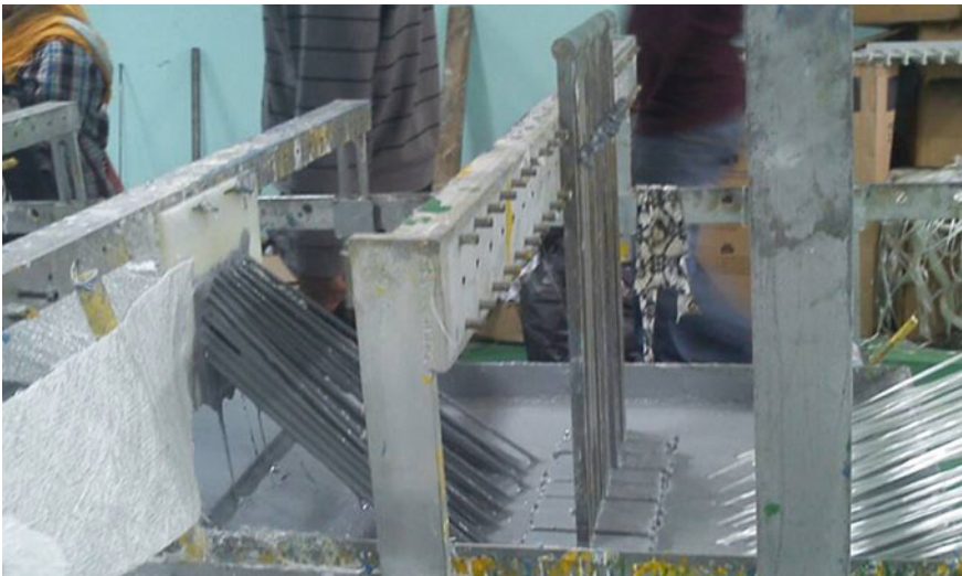
Fig. 1.5 Pultrusion process of glass fibre reinforced epoxy composite rods
