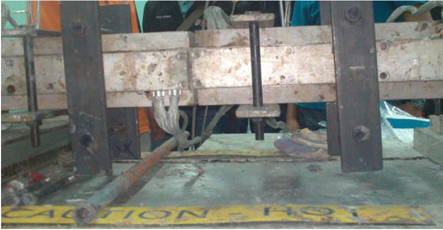
Fig. 6.12 Continuous roving travel through heated die (Courtesy of Innovative Pultrusion Sdn. Bhd., Seremban, Malaysia)
