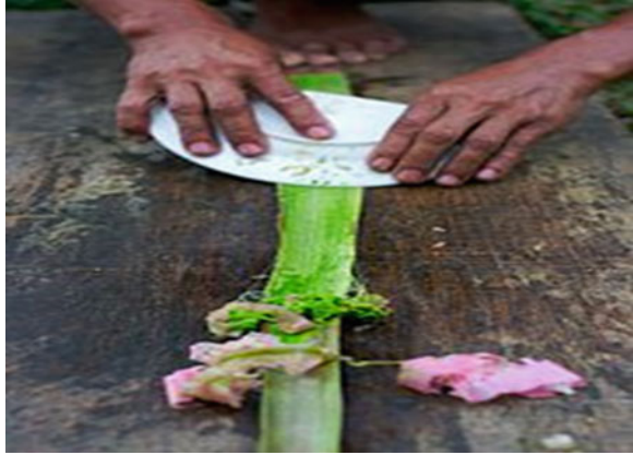
Fig. 2.31 Fibre extraction by scrapping (Courtesy of Dr. Januar Parlaungan Siregar, Universiti Malaysia Pahang)
