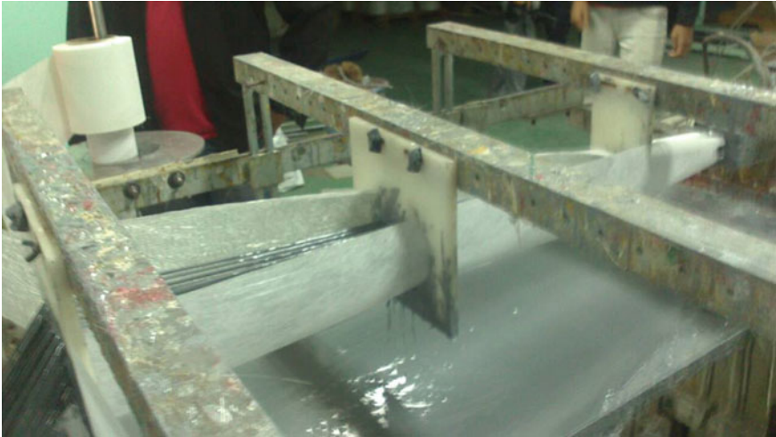
Fig. 6.10 Continuous roving travel through guides toward resin bath and forming station (Courtesy of Innovative Pultrusion Sdn. Bhd., Seremban, Malaysia)
