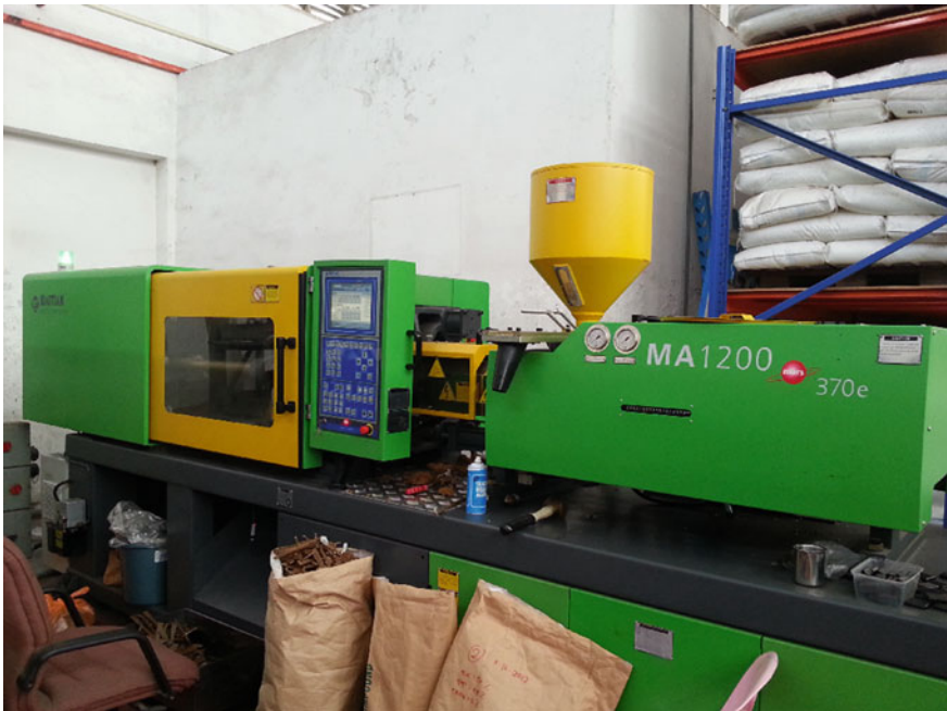
Fig. 6.15 Injection moulding (Courtesy of Mr. Azaman Md Darus, Universiti Malaysia Perlis, Malaysia)
