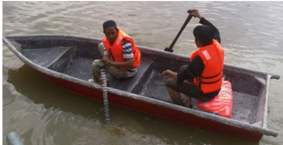
Fig. 7.7 Small boat from hybrid glass-sugar palm composites
