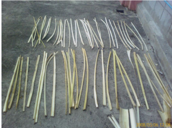
Fig. 2.5 Drying of banana pseudo-stem fibres under the sun
