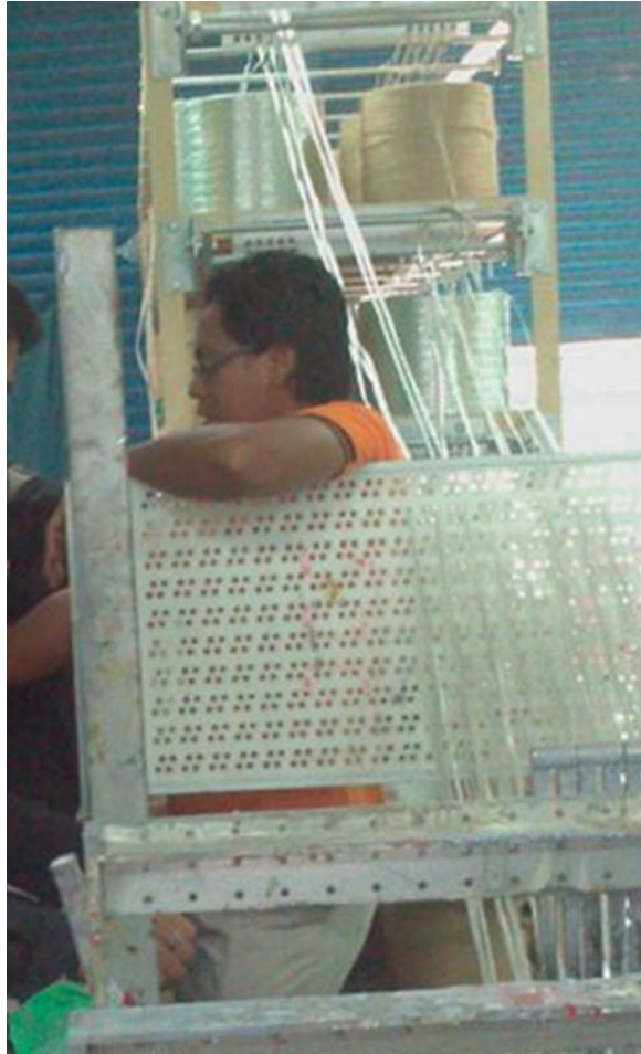
Fig. 6.9 Continuous roving travel from creels toward resin bath (Courtesy of Innovative Pultrusion Sdn. Bhd., Seremban, Malaysia)
