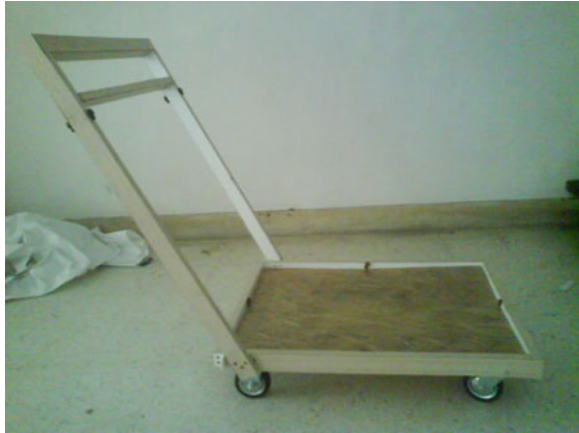
Fig. 7.6 Trolley base from kenaf fibre composites
