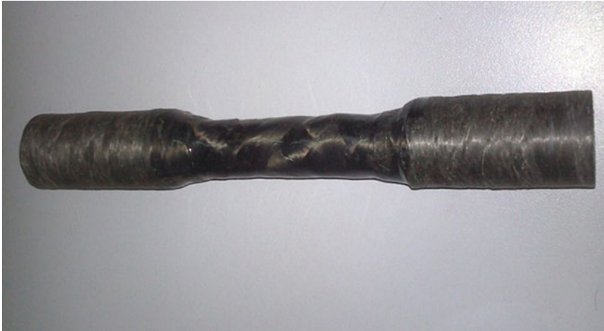
Fig. 1.6 Automotive drive shaft made from filament wound carbon fibre reinforced epoxy composites
