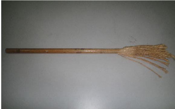
Fig. 7.2 Pultruded rod from kenaf composites
