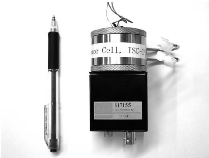
Fig. 14 Impinging jet type CTL-based sensor cell with a photomultiplier module
