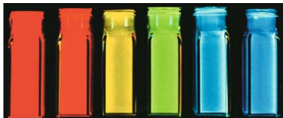
Fig. 15.2. The color of the emission is dictated by the size of the core, as illustrated for a series of highly fluorescent CdSe/ZnS core/shell nanocrystals from the Quantum Dot Corporation. The CdSe nanocrystal core is smallest (18 Å) for blue emitting dots and largest (60 Å) for red emitting dots
