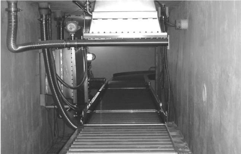
Figure 9-14. A possible configuration of a slat conveyor in the process corridor. A section of the scan horn from the downward-directed beam is shown. (Used with permission of the Titan Corporation.)
