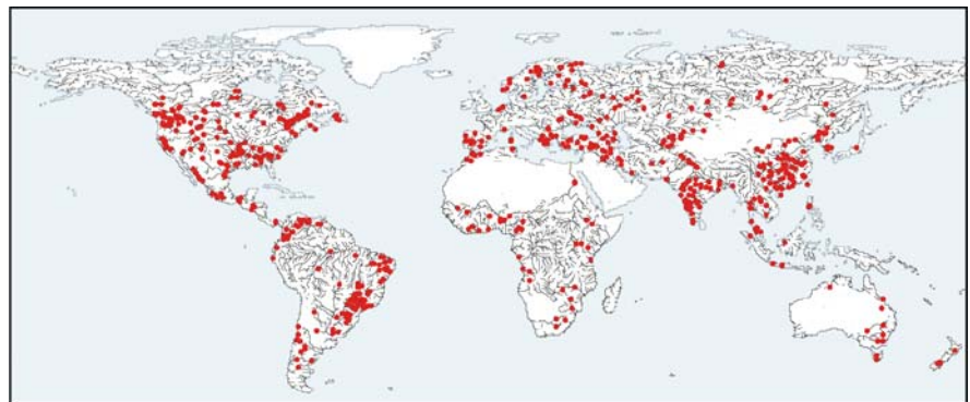
Fig. 2.18. Water fluxes. Distribution of the world's major dams. Between 10.6% and 12.5% of the total annual river runoff ( 42\,650 \text{ km}^3 \text{ yr}^{-1} ) is presently stored behind large dams, mostly created since the 1950s
