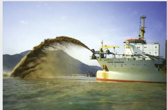
Fig. TB2.10.4. A trailing suction hopper dredger from the Netherlands similar to the type used for the reclamation of the new Hong Kong International Airport in action in Hong Kong. Sand is placed hydraulically using a technique known as rainbowing (© W. W.-S. Yim)
