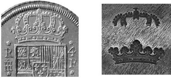
Fig. 12 Coin and punch-block for roller-dies from the Segovia Mint in 1728. The crown is composed of two punches since the vertical extension of the design is severely limited by the curvature of the cylinder. Madrid Mint Museum
