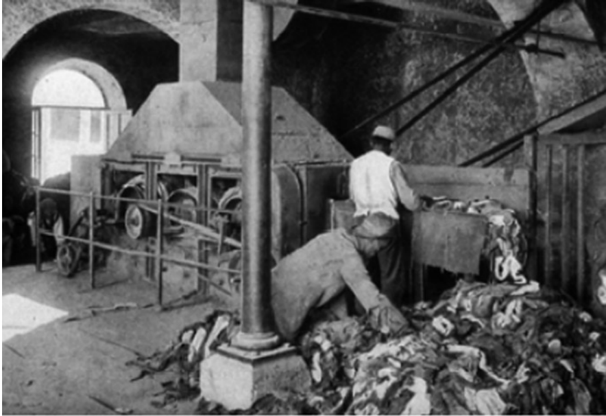
Fig. 12 Smashing machine in the paper mill Fibreno in Isola del Liri (Mancini 2007)
