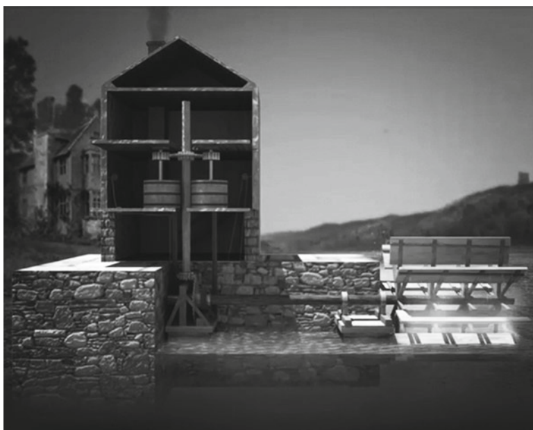
Fig. 21 Water mill with floating waterwheel
