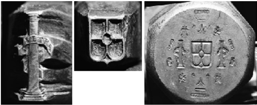
Fig. 16 Punches and punch-block for flat dies made in Madrid in 1770 and sent to the Mint in Potosí, Bolivia. Glenn Stephen Murray Fantom
