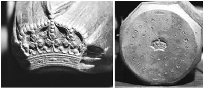
Fig. 13 Punch and punch-block for flat dies made in Madrid in 1770 and sent to the mint in Potosí, Bolivia. The crown is composed of one punch. Glenn Stephen Murray Fantom
