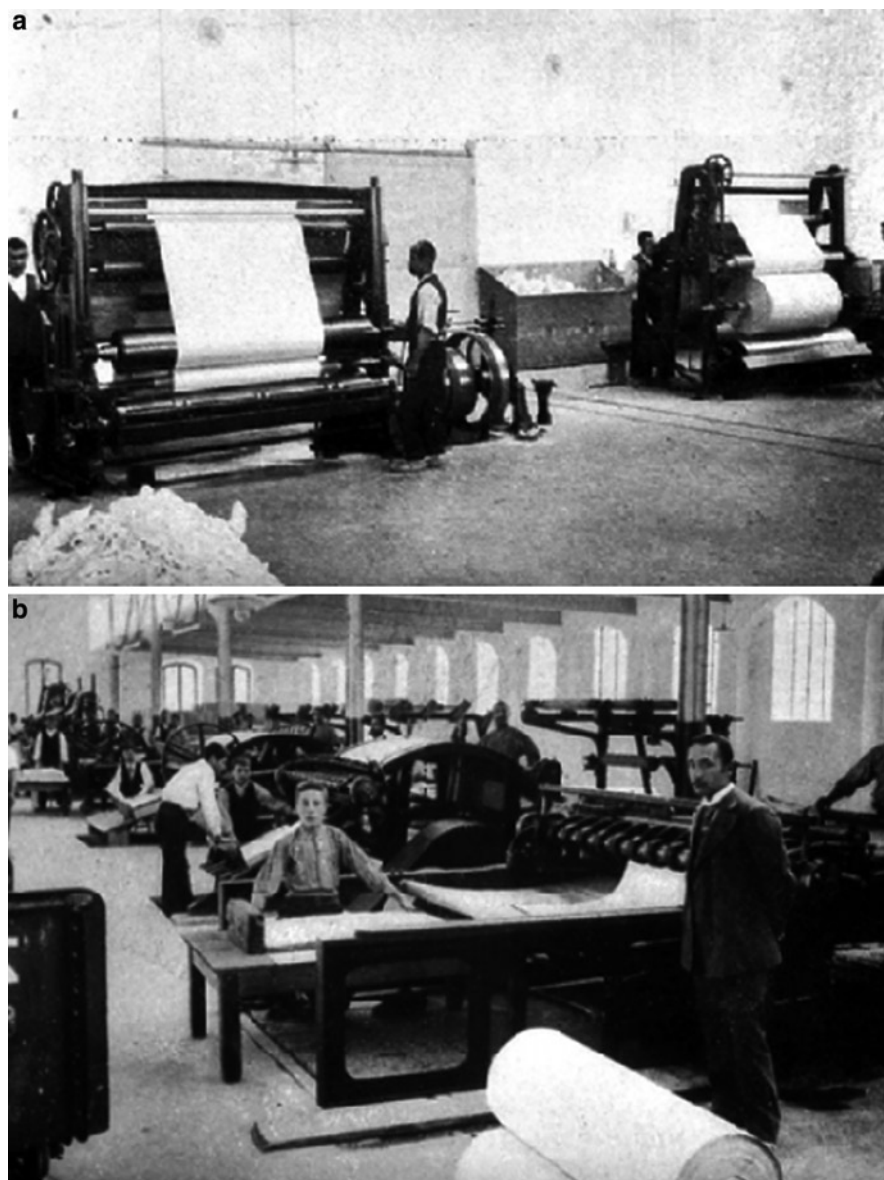
Fig. 15 Machines in the paper mill Cartiera del Liri in Isola del Liri (Mancini 2007): (a) packing machine; (b) cutting machine
