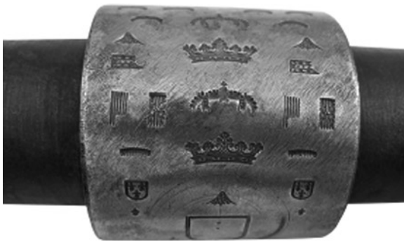
Fig. 14 Punch-block for cylindrical dies from the Segovia Mint circa 1700 – 1730. Madrid Mint Museum
