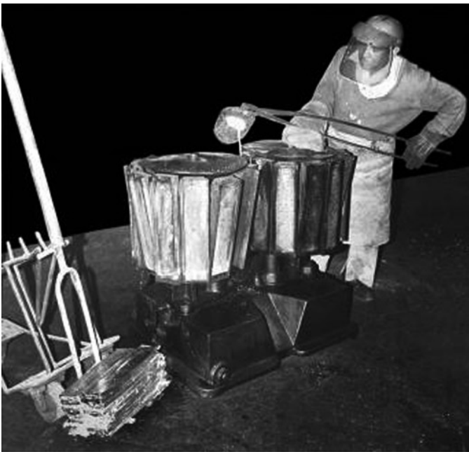
Fig. 45 Pouring of metal into the molds to form the flat ingots which are later rolled into strip. Glenn Stephen Murray Fantom
