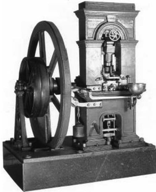
Fig. 40 Modern belt-driven coin press with automatic blank feeder, from the mid nineteenth century. Madrid Mint Museum
