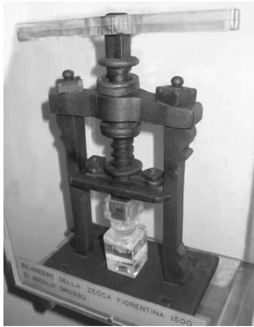
Fig. 25 Blank cutting press from the sixteenth century. Museum of Science and Technology, Milan, Italy
