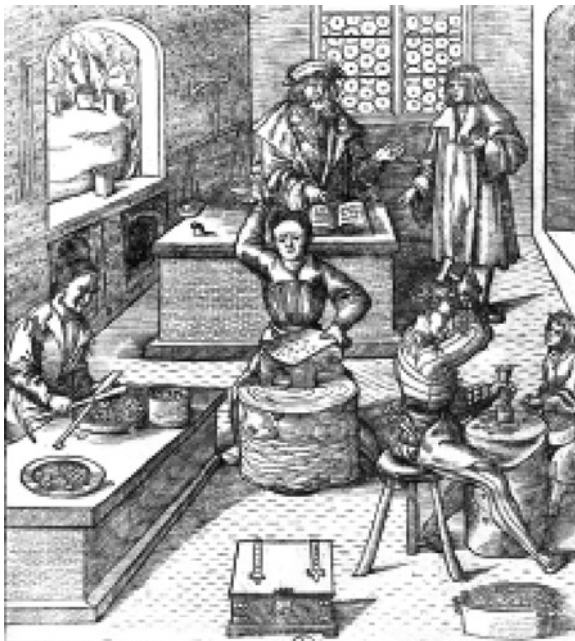
Fig. 18 Sheet pounding, blank cutting and annealing, and coin striking in a non-mechanized hammer mint. National Library, France
