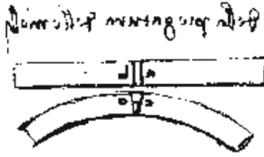
Fig. 5.1 Leonardo da Vinci's understanding of bending of beams
