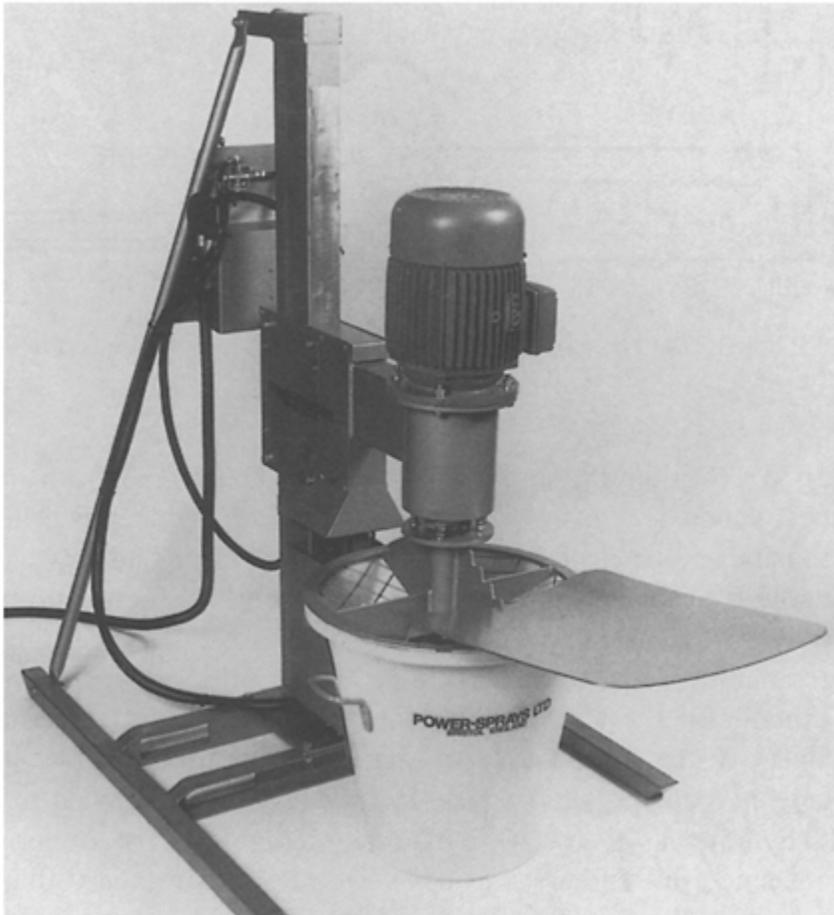
FIGURE 2.8 High shear (1400 rpm) mixer used to prepare mortar prior to adding glass fibers in the premix process (Courtesy of Power-Sprays Ltd.)
