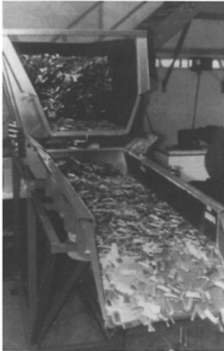
FIGURE 5.10 Integrated system for separating, weighing and batching steel fibers consisting of vibrating feeder silo and vibrating weigh hopper conveyor with variable controlled discharge rate (Courtesy of Skako Ltd.)
