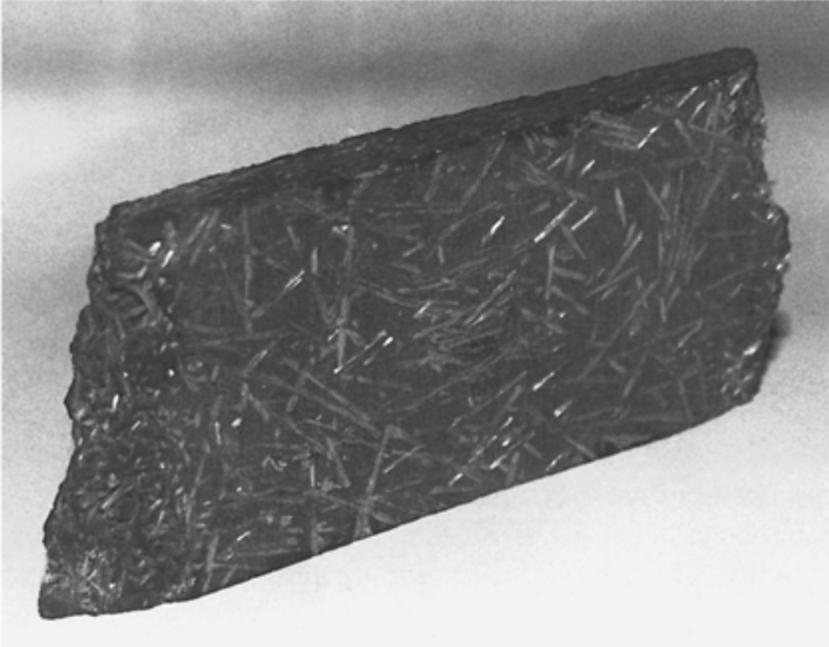
FIGURE 1.1 Glass fiber-reinforced cement
