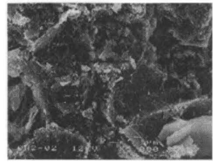
Figure 5 Fines-cement composite with wood chips treated with lime, (lime/wood = 0.5) G = 5000
