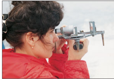
Figure 20.1 Sextants (a) are traditional navigation instruments which have been in use (b) since 1731. The diagram (c) illustrates the use of sextants for position-fixing in good visibility up to a few kilometres from the landmarks. Two sextants are used to measure simultaneously the angles between three landmarks or objects of already-known position – further calculation allows two intersecting position circles to be drawn 6 . This technique can give accuracies of a few metres, but using sextants from the deck of a boat (an unstable platform) requires practice! (d) Lines A, B, and C are known as position lines. Each position line has an associated error which is dependent on the position-fixing system being used. This diagram shows the effect of errors associated with two of the position lines. Instead of the position being defined at a single point, the vessel’s position lies somewhere within the parallelogram. No matter what position-fixing system is used, an error will always be associated with each position line. For high-accuracy positioning at least three position lines are normally used to try and minimise the effect of errors.
