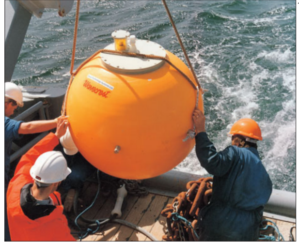
Figure 19.14 A Wavecrest buoy, developed by the Netherlands company Datawell, being deployed. The buoy follows the sea surface and sensors measure the components of acceleration, which, integrated twice, give the wave-height variations. The buoy is moored to the sea bed using a compliant tether – usually a length of thick rubber line – to avoid mooring forces affecting the record. (Courtesy of C. Griffiths, Dunstaffnage Marine Laboratory, Oban, Scotland.)
