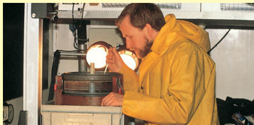
Figure 7.13 The large-volume marine snow catcher, the 'snatcher', for collecting undamaged samples of the aggregates. (a) The entire device just prior to deployment from RRS Discovery. (b) The lower chamber of the 'snatcher' in the cold laboratory on board ship. Aggregates are being collected from the base of the chamber using a wide-bore pipette to avoid damage. The lights are directed through the transparent sides of the chamber for ease of collection.
