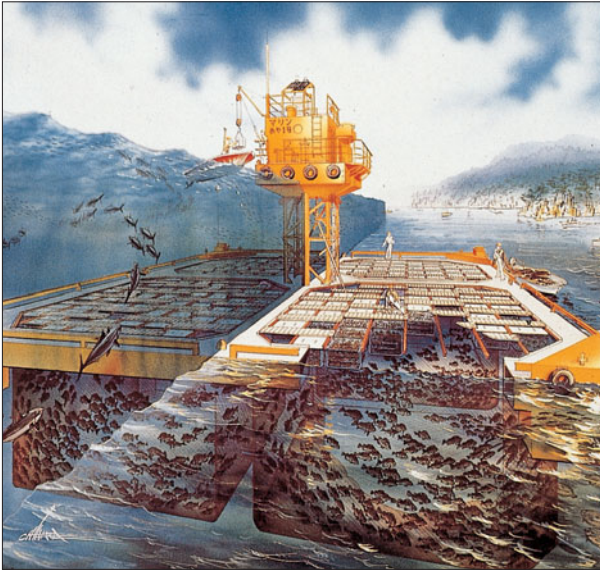
Figure 21.12 (a) Development by the Japanese Marine Science and Technology Centre (JAMSTEC) of an artificial sea floor (20 x 20 m), which can be raised to the surface (right) and lowered below the surface (left) to and from its working depth of 4 m; it forms a platform for growing abalones, and its tanks contain black rock-fish. (b) On the prototype in Ryohri Bay, Japan, the abalone are fed with kelp and measured at the surface once a week. (© Mineo Okamoto, JAMSTEC, Japan.)
