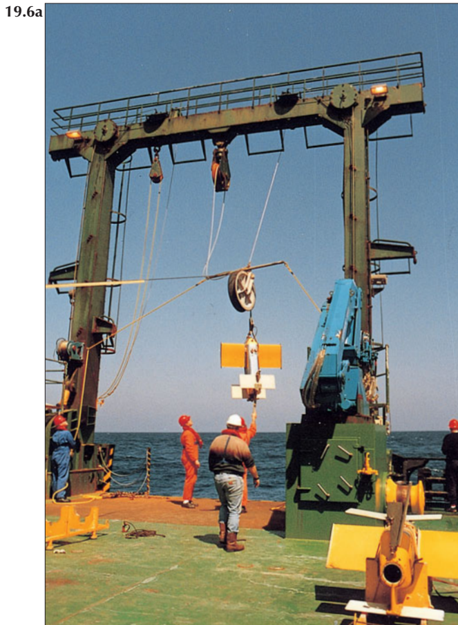
Figure 19.6 Towed vehicles do away with the need for the vessel to stop and lower instruments. The SeaSoar undulator travels from the surface to 500 m depth in a horizontal distance of 2 km at a ship speed of 9 knots (about 4.5 m/s). It carries CTDs and other physical, chemical, and biological instruments to measure the structure of the upper ocean (see, for example, Figure 4.10 ). (a) Deployment through the stern ‘A’ frame of RRS Charles Darwin is straightforward in calm seas, but can be difficult in a gale (a spare vehicle is in the right foreground). (b) The vehicle being deployed – SeaSoar’s ability to carry several instruments makes it especially valuable for research spanning more than one discipline. Increasingly, the vehicle is used to make measurements for biological oceanographers, including ocean colour, phytoplankton pigments, and zooplankton counts using optical and acoustic sensors.
