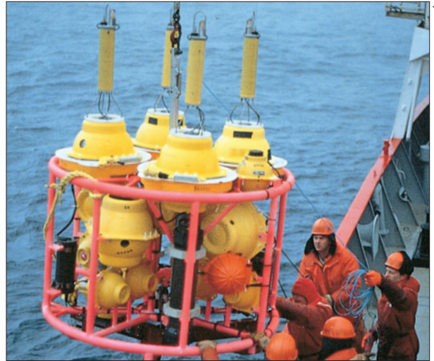
Figure 19.18 Sea-level changes of centimetres can be observed from the deep-ocean floor by the MYRTLE package. Designed for operation over 5 years, MYRTLE releases data 'podules' to the surface, where, as they drift, they telemeter data to the laboratory via ARGOS satellites. The package shown here is being deployed on the continental slope off the Antarctic Peninsula, the southern boundary of Drake Passage. With another MYRTLE package on the northern slope off South America, the slope of the sea level between the two sites provides a measure of the transport of water through the Drake Passage by the Antarctic Circumpolar Current, and of its variability (see Chapter 4). (Courtesy of Proudman Oceanographic Laboratory, Bidston, UK.)
