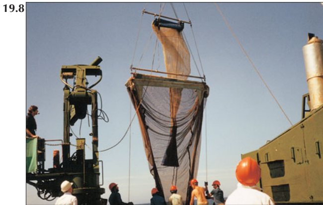
Figure 19.8 The Rectangular Midwater Trawl (RMT) 1+8 acoustically controlled mid-water net system consists of a pair of rectangular trawl nets within a single frame. The outer net has an opening area of 8 m 2 with a mesh of 4.5 mm to catch micronekton, the inner net with an opening area of 1 m 2 with a finer mesh (320 µm) is for plankton. Acoustic commands from the ship control a mechanical release gear to open and close the nets. Data on temperature, depth, speed and distance travelled, and net position are telemetered acoustically to the ship. (Courtesy of SOC.)
