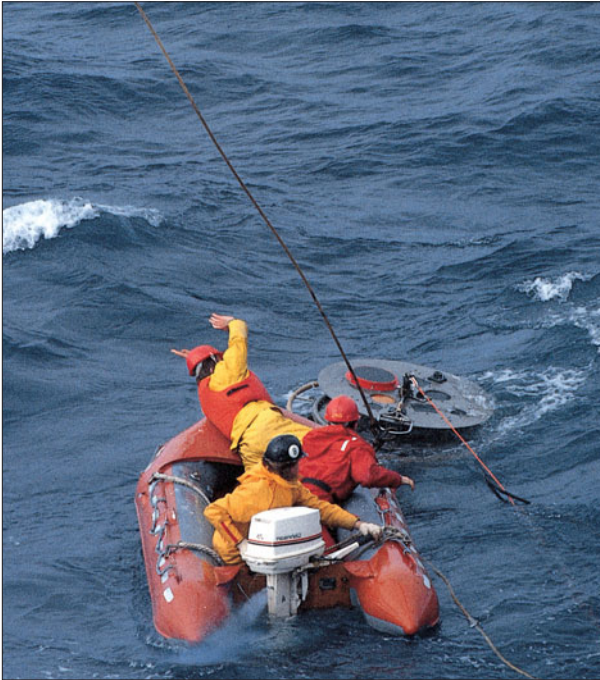
Figure 19.29 A hydrophone array, used to ‘listen to’ and track the motion of breaking waves, which play an important part in the transfer of momentum and gases between the air and the sea (see Chapter 2), being recovered using a Zodiac inflatable boat. Recovery of equipment at sea is often a difficult and potentially dangerous operation, requiring careful attention to stringent safety precautions. For further details of the equipment and its use, see Farmer and Ding 1 . (Courtesy of Dr D. Farmer, Institute of Ocean Sciences, Sidney, British Columbia, Canada.)
