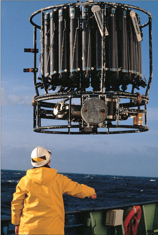
Figure 19.2 A deep-ocean hydrographic instrument package consisting of a CDT, a 24 x 10 litre-bottle rosette multisampler, fluorometer, and transmissiometer. (Courtesy of S. Hall, SOC.)
