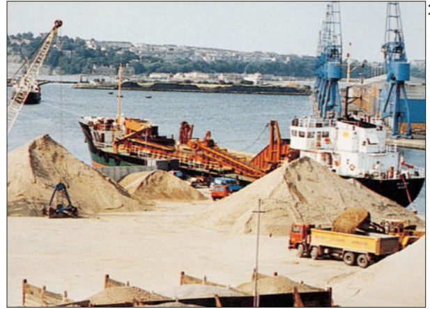
Figure 21.29 Piles of sand and gravel from offshore on the quayside awaiting distribution. (© United Marine Dredging Ltd, England.)
