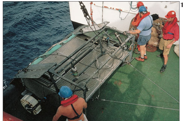
Figure 19.9 The epibenthic sledge is designed to skim over the surface of the sea bed and collect the organisms living on the sea floor, immediately above it, and in the upper few centimetres of the sediment. An acoustic pinger indicates when the sledge has reached bottom, when the opening–closing mechanism has operated, and when the sledge leaves the bottom. Cameras and electronic flash may be mounted on the sledge to provide images of the nature of the bottom and to give some indication of the efficiency of the net in capturing animals. (Courtesy of SOC.)
