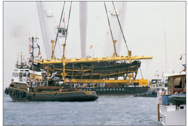
Figure 18.8 The Mary Rose , a Tudor warship sunk on the South coast of England in 1547, was buried in mud with one side virtually missing. From measurements and drawings made by divers excavating inside the hull and burrowing underneath it, a cradle was constructed to exactly fit and support the fragile structure as it was lifted from the sea bed. At no time, before it was lifted out of the mud, could the entire ship be seen or measured.
