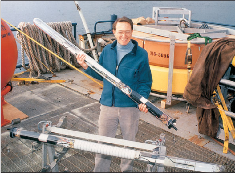
Figure 19.22 A WOCE-style RAFOS float being held before deployment on R/V Knorr . This version of the float was recently developed by the University of Rhode Island and the Woods Hole Oceanographic Institution, and is manufactured by Seascan Inc. RAFOS floats are ballasted to be neutrally buoyant at a pre-selected depth, where they drift for as long as several years, showing the water motions (see Chapters 3 and 4). The floats receive acoustic signals from moored sound sources, record the times of arrival so that their position can be determined, and (at the end of their mission) surface and transmit the data, including temperature and pressure, back to the laboratory via the ARGOS satellite system. (Courtesy of Dr T. Kleindinst, Woods Hole Oceanographic Institution, Woods Hole, Massachusetts, USA.)
