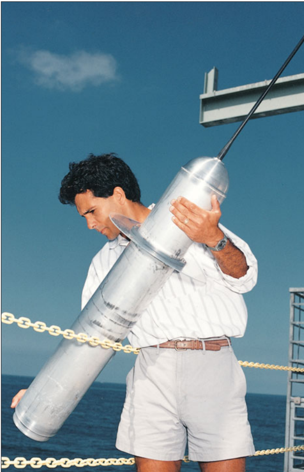
Figure 19.23 An ALACE float, showing the satellite telemetry and location antenna. Instead of obtaining position fixes from moored sound sources, the ALACE float periodically increases its buoyancy and rises to the surface every 20 days. There, by using the ARGOS platform location and data transmission satellite system, the ALACE float can be located and data sent to shore before the float returns to its pre-set depth. The major challenge in designing the ALACE float was to devise a reliable, high-efficiency buoyancy control system that could function at ambient pressures of up to 200 bar. The buoyancy change is performed by changing the effective volume of the float. An electrically driven hydraulic pump moves oil from a reservoir internal to the float to an external bladder. An example of the float tracks is shown in Figure 3.13 . (Courtesy of Dr R. Davis, Scripps Institution of Oceanography, La Jolla, California, USA.)
