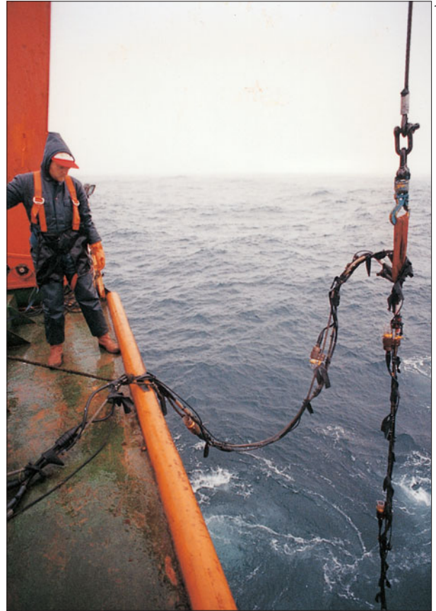
Figure 19.10 A thermistor chain (a) laid out under cover before deployment, and (b) being deployed. This chain of thermistors to measure the thermal structure of the upper ocean is 400 m long and consists of 100 sensing ‘pods’, each providing a measure of temperature, and 28 measures of pressure so that the depth of the measurements are well-established. A 2 tonne sinker weight keeps the chain near-vertical under tow at a speed of 4 knots (about 2 m/s). The chain uses digital data communication and contains only six wires, two for power supply, two for data, and two for control. Sampling the 100 pods takes only 0.9 s. This particular chain has been used on 14 ocean measurement surveys, and more than 30 weeks of continuous data have been collected, comprising some 38,000 km of track. Much of the work has been directed toward the detection and tracking of fronts and eddies in the area between Iceland and the Faeroes, where waters of the North Atlantic meet those of the Norwegian Sea. (Courtesy of Dr J. Scott, Defence Research Agency, Dorset, UK.)
