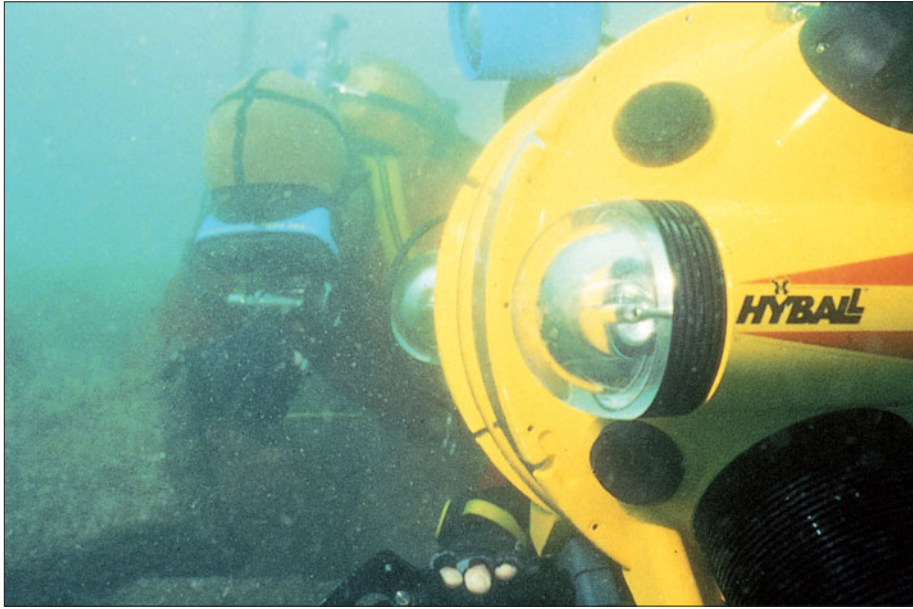
Figure 18.2 Divers support remotely operated equipment – each have their uses. While the ROV is not adversely affected by cold or pressure and can work indefinitely, the diver is far more manoeuvrable, has more dexterity, and, above all, can think.
