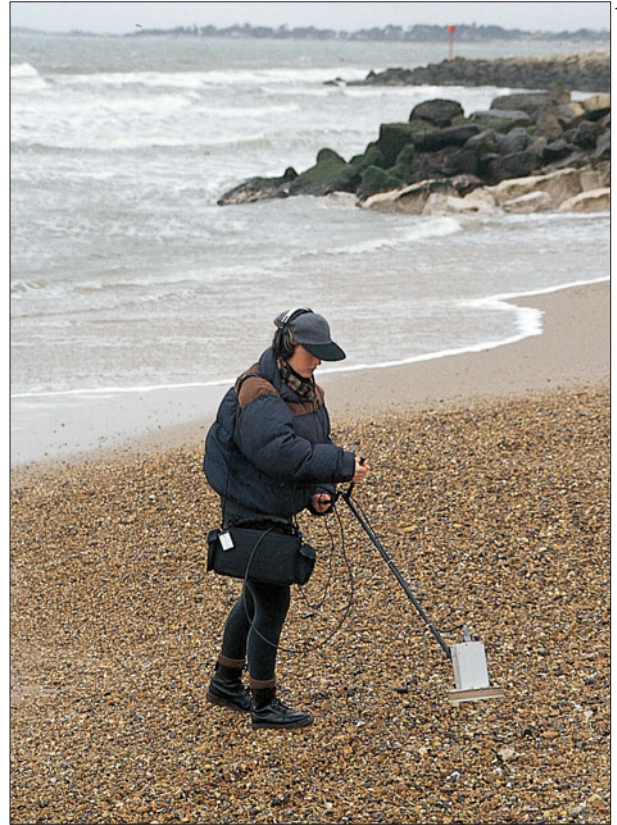
Figure 19.24 The ‘electronic pebble’ is a tracer developed to monitor the mobility of shingle on beaches. (a) The system comprises synthetic pebbles consisting of a battery-operated circuit (A, B, and C) encapsulated in resin (D), which emits a coded train of magnetic pulses (scale bar, 0–10 cm). These are placed on the beach at low tide and can then be detected and decoded by a portable receiver (b) or a towed receiver (c) when in close proximity. Their movement indicates the motion of similar pebbles. (Courtesy of Dr M. Workman, SOC.)
