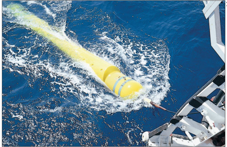
Figure 20.12 (a) The GLORIA side-scan vehicle during deployment from its dedicated launch cradle. The vehicle is 7.75 m in length and weighs approximately 2 tonnes in air, but is neutrally buoyant in sea water. It is towed at a speed of between 8–10 knots. (b) GLORIA 6.5 kHz side-scan image showing a linear chain of submarine volcanoes in the Pacific Ocean, west of San Francisco (scale bar is 20 km) – strong sonar targets are white, acoustic shadows are black (note this is opposite to those in Figure 20.11 ).
