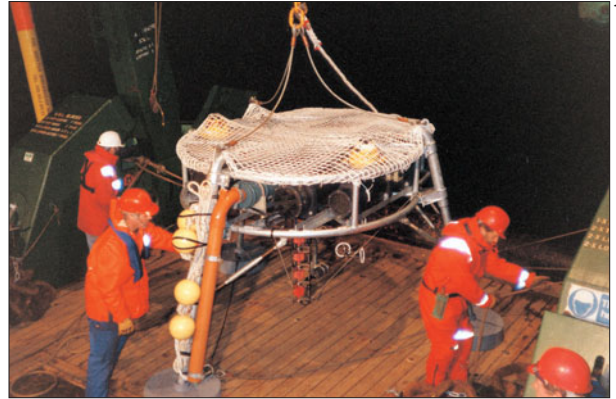
Figure 19.17 Work on research vessels proceeds through the night – here deploying the Sediment Transport and Boundary Layer Equipment (STABLE) benthic instrument platform with current and high-frequency acoustic sediment transport sensors. (Courtesy of J Humphrey, Proudman Oceanographic Laboratory, Bidston, UK.)
