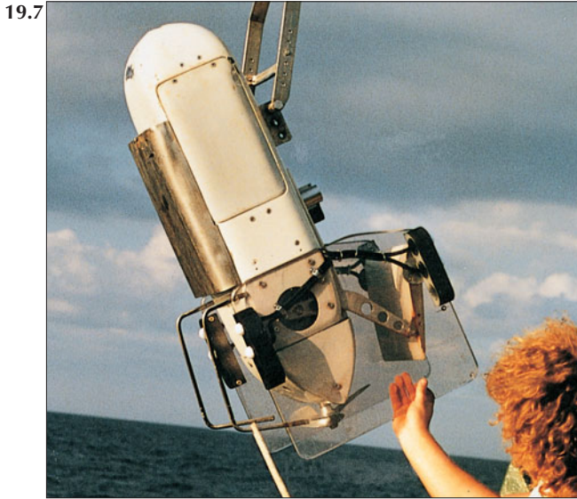
Figure 19.7 Introduced in the early 1970s, the UOR – known commercially as the Aquashuttle – can be towed from ships of opportunity at speeds of up to 10 m/s. The vehicle can either be self-contained, following pre-set undulations and storing data internally, or it can be controlled from the ship through a conducting cable to give real-time data. It can be launched by one person and can record its data internally. It is ideally suited for deployment by non-experts on merchant ships, so extending the geographical coverage of data collection beyond the tracks of research vessels in a most cost-effective way. (Courtesy of Plymouth Marine Laboratory, Plymouth, UK.)
