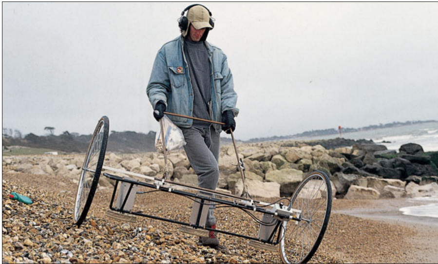
Figure 19.24 The ‘electronic pebble’ is a tracer developed to monitor the mobility of shingle on beaches. (a) The system comprises synthetic pebbles consisting of a battery-operated circuit (A, B, and C) encapsulated in resin (D), which emits a coded train of magnetic pulses (scale bar, 0–10 cm). These are placed on the beach at low tide and can then be detected and decoded by a portable receiver (b) or a towed receiver (c) when in close proximity. Their movement indicates the motion of similar pebbles. (Courtesy of Dr M. Workman, SOC.)
