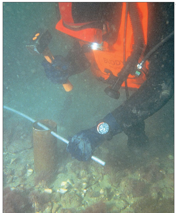
Figure 18.9 A diver collects core samples (for infaunal analysis) of a known volume from a stony sea bed, which are not easily obtained remotely. A metal tube is hammered into the sea bed to a known depth. The tube is then dug out and capped at each end for recovery. If necessary, a compass can be used to determine the tube's magnetic orientation and it can be kept upright as it is brought to the surface. Several replicates are usually collected to ensure a representative sample.
