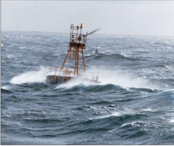
Figure 19.13 A surface meteorology buoy, with anemometers (for mean wind speed and direction), sea and air temperature sensors, a 3 m path acoustic current meter, a buoy motion package (to give wave height and directional spectrum), and radio and satellite data telemetry (see Chapter 2 for a discussion of the way the atmosphere affects the ocean). (Courtesy of A. Hall, SOC.)
