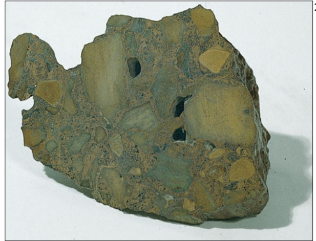
Figure 21.31 Phosphatic limestone with a P_2O_5 content of around 15–18% dredged from the continental shelf off Morocco (maximum dimension 12 cm). This example is a conglomerate of pebbles of phosphatised limestone and phosphorite set in a phosphorite matrix, in which are embedded dark green to black, sand-sized grains of the iron–potassium aluminosilicate mineral glauconite. The rock is believed to have formed in Miocene times. Being solid, rather than pelletal, and having a moderate P_2O_5 content, it is a rather low-grade resource of fertiliser phosphate, so is uncompetitive with the extensive high-grade pelletal phosphorite deposits mined onshore in Morocco. Miocene glauconitic conglomeratic phosphatic limestones like this are also common off South Africa and California. All three sites are today washed by nutrient-rich upwelling currents; similar, but richer, currents may have prevailed at these sites during the Miocene in response to a global reorganisation of oceanic nutrients. (Photo, M. Conquer; © IOSDL.)
