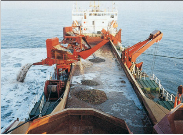
Figure 21.28 Gravel being pumped aboard an offshore dredger. (© United Marine Dredging Ltd, England.)
