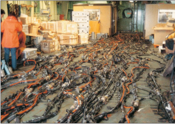
Figure 19.10 A thermistor chain (a) laid out under cover before deployment, and (b) being deployed. This chain of thermistors to measure the thermal structure of the upper ocean is 400 m long and consists of 100 sensing ‘pods’, each providing a measure of temperature, and 28 measures of pressure so that the depth of the measurements are well-established. A 2 tonne sinker weight keeps the chain near-vertical under tow at a speed of 4 knots (about 2 m/s). The chain uses digital data communication and contains only six wires, two for power supply, two for data, and two for control. Sampling the 100 pods takes only 0.9 s. This particular chain has been used on 14 ocean measurement surveys, and more than 30 weeks of continuous data have been collected, comprising some 38,000 km of track. Much of the work has been directed toward the detection and tracking of fronts and eddies in the area between Iceland and the Faeroes, where waters of the North Atlantic meet those of the Norwegian Sea. (Courtesy of Dr J. Scott, Defence Research Agency, Dorset, UK.)
