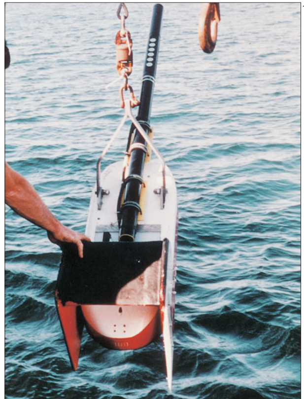
Figure 19.11 The Lightfish is an instrument to measure multispectral reflectance at high spatial resolution. There are six sensors pointing up and down, the six white ports in the upper black bar, within which are mounted the irradiance sensors sampling at 410, 440, 490, 520, 550, and 670 nm. It is towed just below the water surface from a ship, collecting data from ocean transects which can be compared with observations from airborne or satellite sensors; this provides ‘ground-truth’ calibrations of these sensors for ocean colour estimates, which can be related to the near-surface distribution of phytoplankton (see Chapter 14). Data are logged onto a ship-board computer, together with other relevant data such as temperature, fluorescence, and transmittance. (Courtesy of Dr A. Weeks, SOC.)
