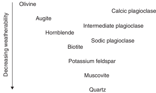
Figure 8.2. The Goldich weathering sequence based on observations of the sequence of their disappearance in soils (Goldich, 1938).
