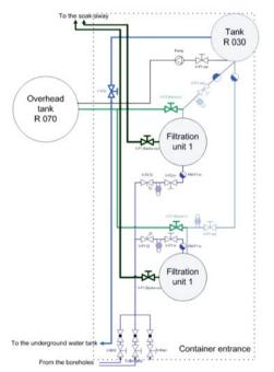
Picture 9: Schematic representation of the groundwater treatment plant (top view)
