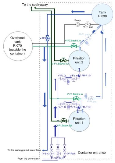
Picture 17: Schematic representation of the treatment plant - flow directions during the filtration process (top view)
