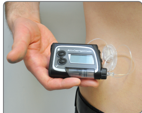
Figure 3.7 Insulin pump with plastic-giving set and subcutaneous needle to allow delivery of the insulin
