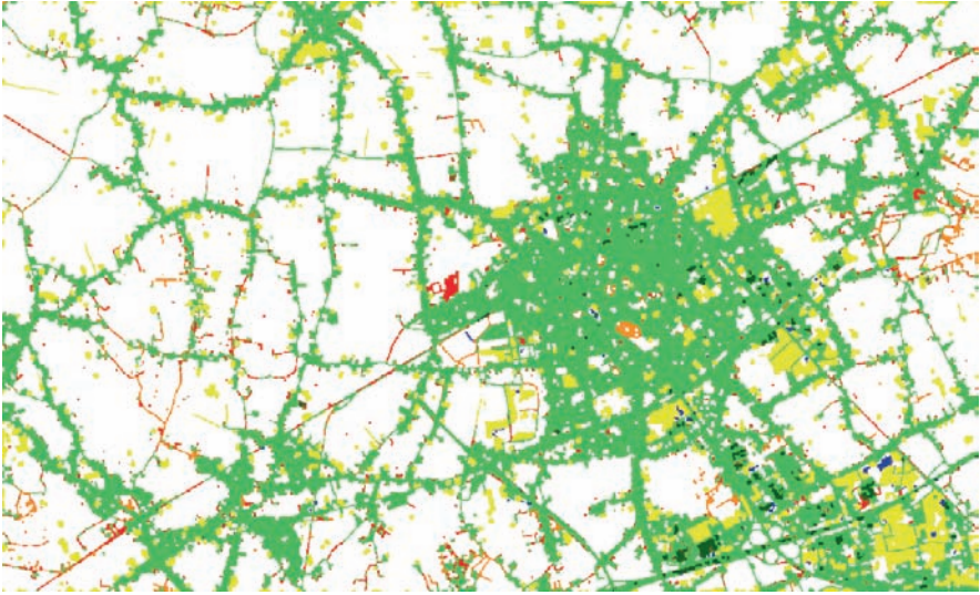
Fig. 9.3 RMA change map of St. Niklaas (Belgium) using NDVI and texture detection. Bright green: no change (NDVI + texture); dark green: no change (NDVI only); red: missed objects or database errors (NDVI + texture); orange: missed objects in forest (NDVI + texture); yellow: changes or false alarms (NDVI + texture); blue: false alarm or changes detected (NDVI only); white: no change (NDVI + texture)
