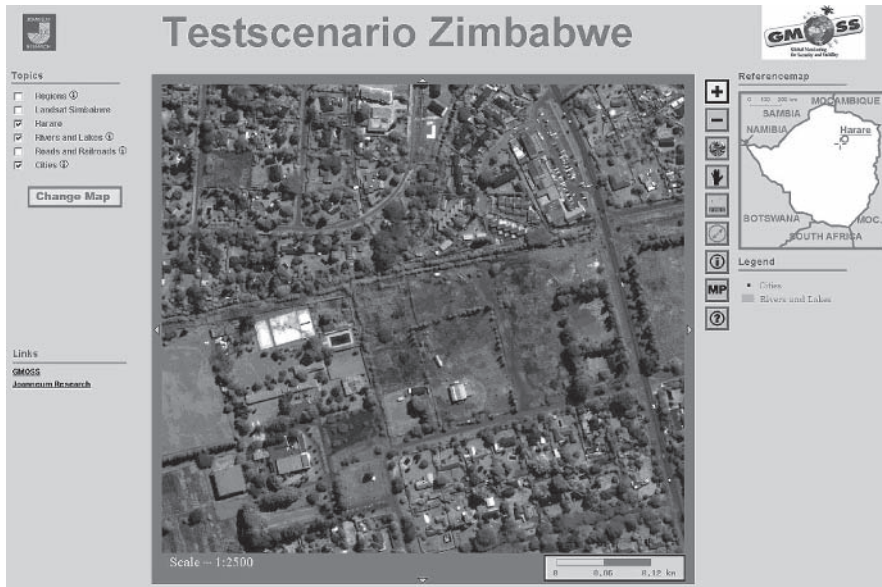
Fig. 10.8 WebGIS client for the test case Zimbabwe showing the city of Harare. Background: Quickbird image, pan-sharpened image with 0.6m ground resolution (Courtesy of JR)
