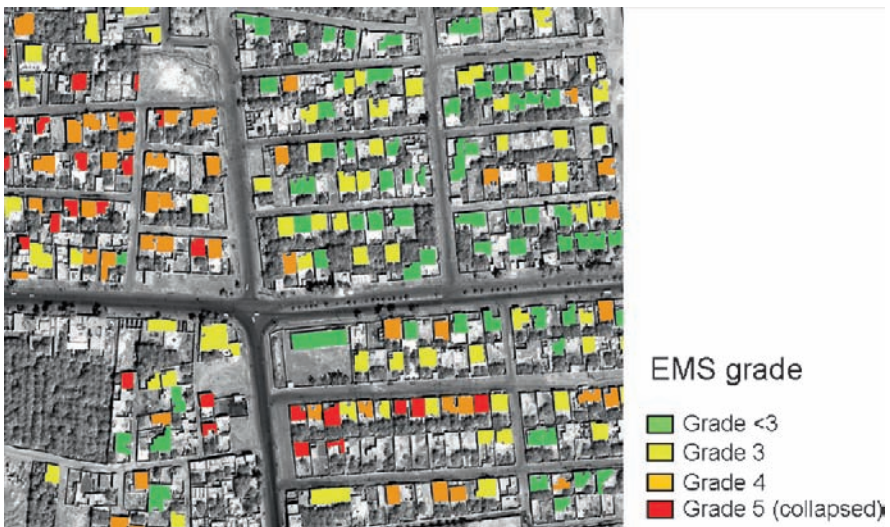
Fig. 16.5 Reference damage database used for roof segmentation and performance evaluation
