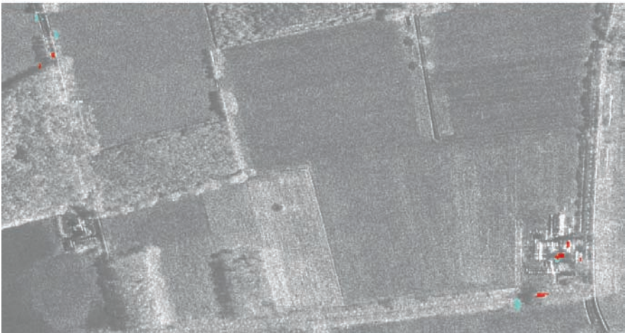
Fig. 9.5 (a) Changes in Intermap AeS-1 SAR images of Borculo (The Netherlands), detected using a hybrid change detection method. Detected are relocated machines and a water tank
