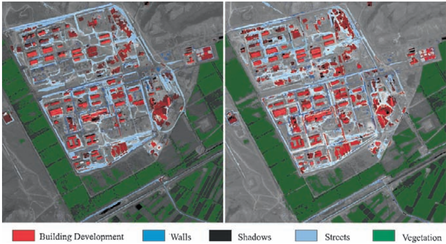
Fig. 12.7 Object-oriented classification of the 2002 (left) and 2003 (right) QuickBird images over Esfahan Nuclear Fuel Research and Production Centre (NFRPC)
