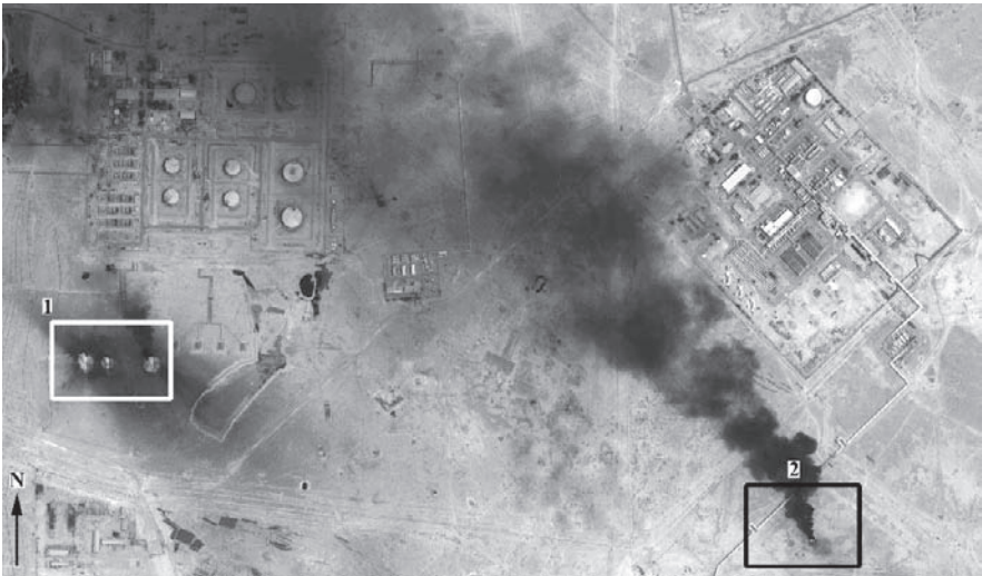
Fig. 13.8 This shows an enlarged section of oil fields at 1 and 2 from Fig. 13.12. Three oil wells are clearly resolved at 1 . This image has a 2m resolution ( http://www.google.co.uk/ and http://maps.google.com/maps )
