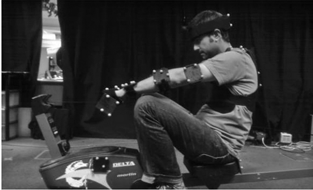
FIGURE 5.4 Upper body motion capture using clusters of markers attached to body landmarks.
