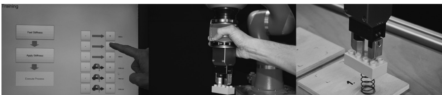
FIGURE 16.5 Main task steps: Setting parameters on touch screen (left), haptic feedback by touch (center), and executing (i.e., compressing spring through parameterized compliance or target point) (right).
