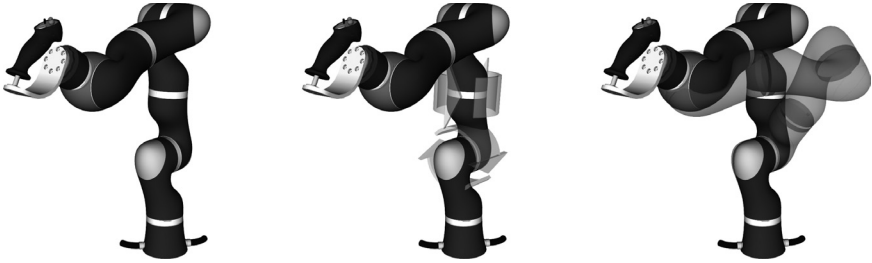
FIGURE 16.2 The light-weight robot (LWR) in a singular situation, and the different kinds of visual pointers; left: no pointer; center: rotating arrows; right: transparent robot.
