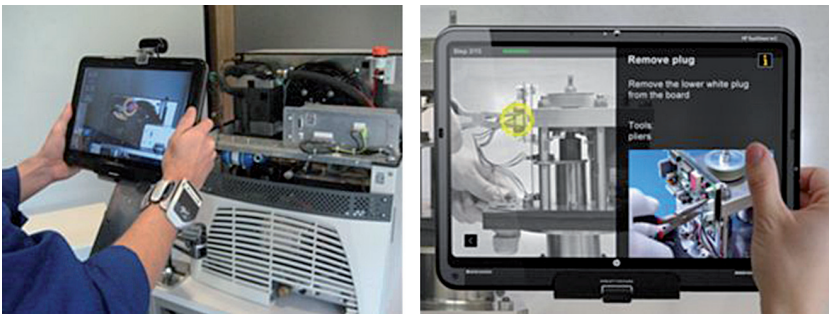
COLOR FIGURE 15.4 IMA-AR platform. Left: The trainee interacts with the IMA-AR platform using a tablet PC that acts as a see-through device; additional haptic feedback is presented via a vibrotactile bracelet. Right: The interactive training application running on the tablet PC.
