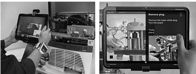
FIGURE 15.4 (See color insert.) IMA-AR platform. Left: The trainee interacts with the IMA-AR platform using a tablet PC that acts as a see-through device; additional haptic feedback is presented via a vibrotactile bracelet. Right: The interactive training application running on the tablet PC.
