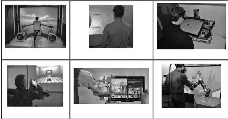
FIGURE 3.1 Six multimodal virtual reality platforms allowing the acquisition and transfer of perceptuo-motor skills in the domains of sports (rowing), entertainment (juggling), surgery (maxillofacial), rehabilitation (upper-limb), industrial maintenance (assembling/disassembling), and programming by demonstration (prototyping).
