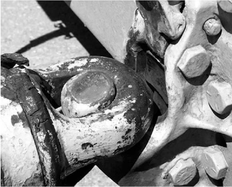
Figure 4.6 Typical trailer hook in a coupler ring on a dolly to allow a tractor-trailer set to pull a second or third trailer. The constraining latch is raised and the compression pad is retracted for visualization purposes. Without the compression pad in place, the space between the pin and tongue ring would be a potential source of slack-action impact.
