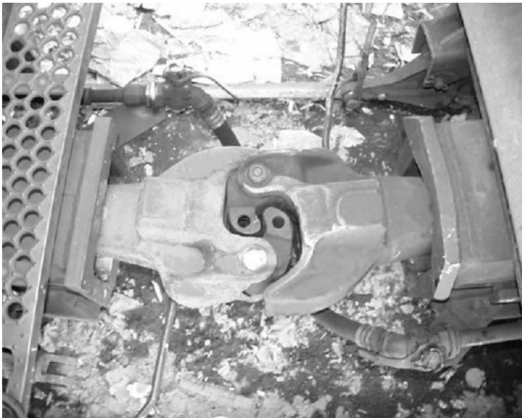
Figure 4.7 Typical train car couplers. The space provides a source for potential slack-action impact. Couplers attached to their cars using a properly-maintained drawbar cushioning apparatus tend to modify the impact from slack action. (Personal communication, Robert Hitson, 18 Dec 2000).
