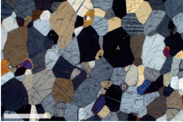
Fig. 4.14 A well-equilibrated microstructure seen in a bytownite-edenite gneiss from Sittampundi, Madras (ample 87975 from the Harker Collection). Note the generally smoothly curved grain boundaries and the \sim 120^\circ dihedral angles developed at all three-grain junctions. The amphibole grain marked with an asterisk shows two faces that are parallel to the \{110\} cleavages, suggesting some anisotropy of interfacial energies. Crossed polars. Scale bar is 1 mm long. The grain marked A is bounded by faces that are concave outwards, whereas that marked B is bounded by faces that are convex outwards. This means the grain A will grow at the expense of grain B during normal grain growth
