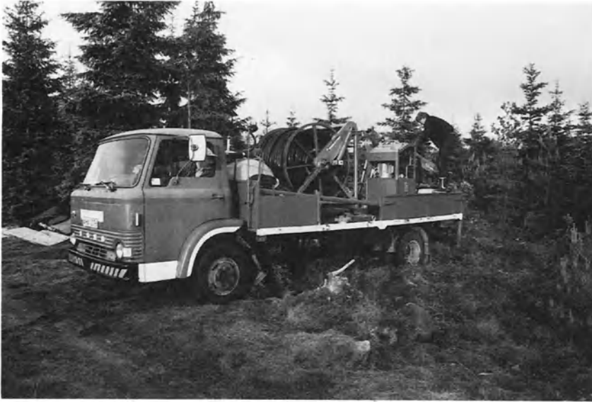
Fig. 4.5 Photograph of first-generation hydrofracturing field truck at Luleå University of Technology, Sweden.
