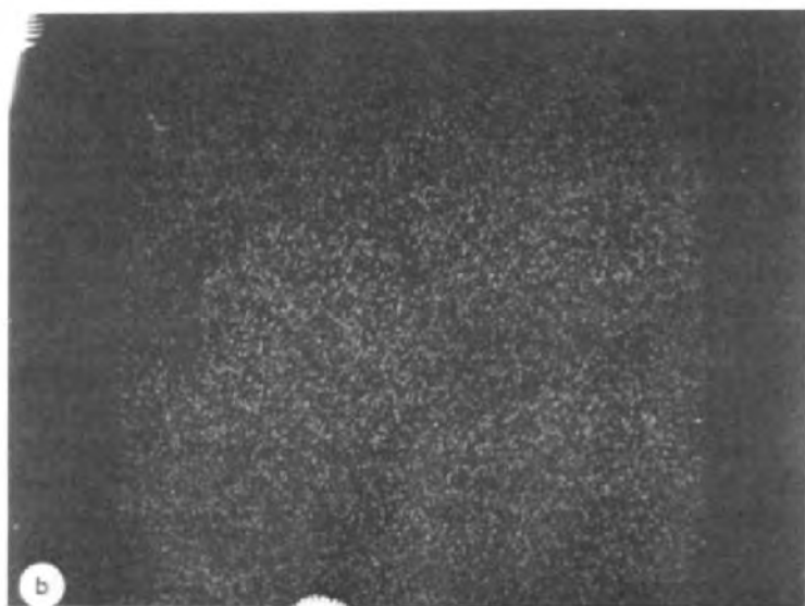
Fig. 7b. Electron microprobe seam at 15 kv, 30 nano amps of a portion of the above field containing pyrite grains set in matrix of silicate minerals. Width of field of view = 0.3 mm (see text for details).
