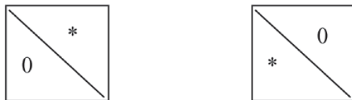
Fig. 2.1-14 Upper (left) and lower (right) triangular matrices; elements in region, marked by 0, are all zero; elements, marked by *, can be non-zero; elements in diagonal are non-zero
