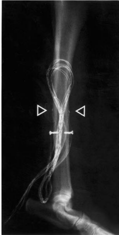
FIGURE 8.2 Radiograph showing two triple 45° rosette strain gauges attached to the cranial surface (left arrow) and caudal surface (right arrow) of a dog tibia. The epoxy resin flanges are approximately 2.5 cm away from each gauge and are screwed into the bone cortex to serve as strain relief.
