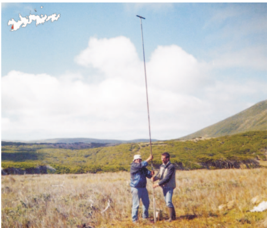
Fig. 7.3 Sampling with a Russian corer (Photo: Ponce 2003)
