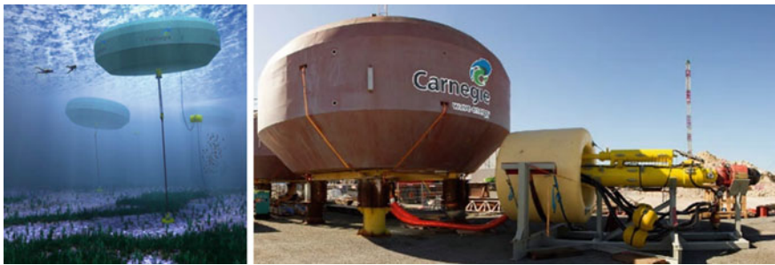
Fig. 16 Carnegies CETO . A submerged tether moored point absorber [33]
