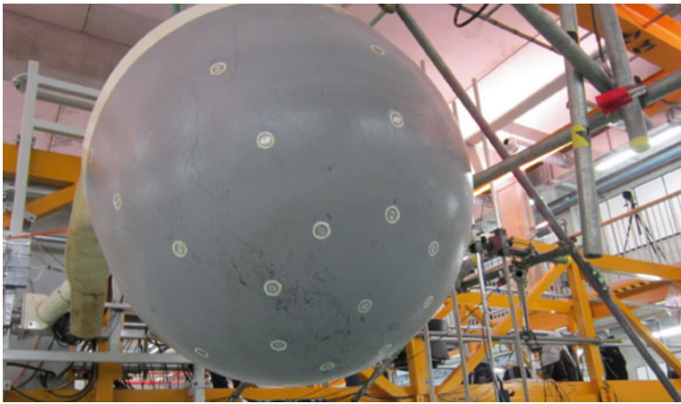
Fig. 18 Picture of a floater of the Wavestar WEC being experimentally tested for wave loads. Courtesy of Wavestar
