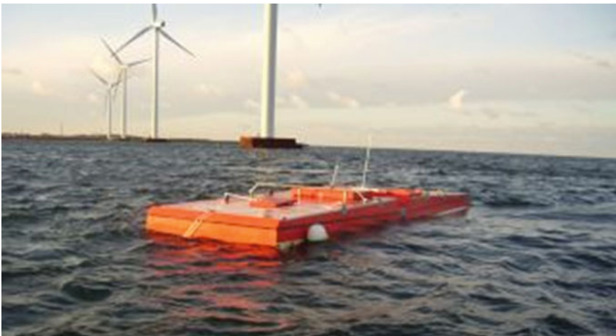
Fig. 10 Crestwing , at a scale of 1:5, tested near Frederikshavn during autumn 2011 [28]
