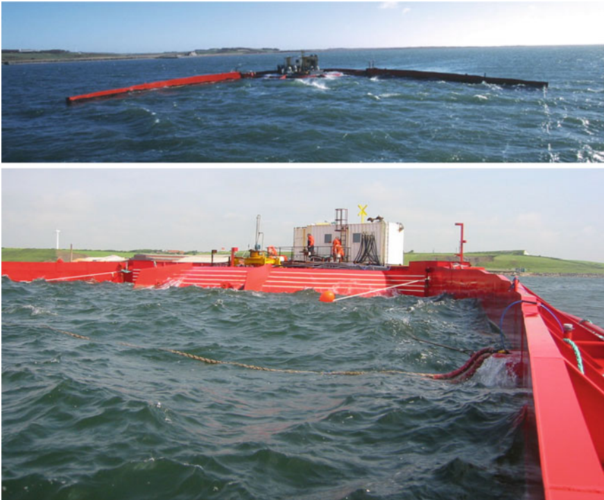
Fig. 24 Wave Dragon 1:4.5 scale grid connected prototype tested in Nissum Bredning, Denmark
