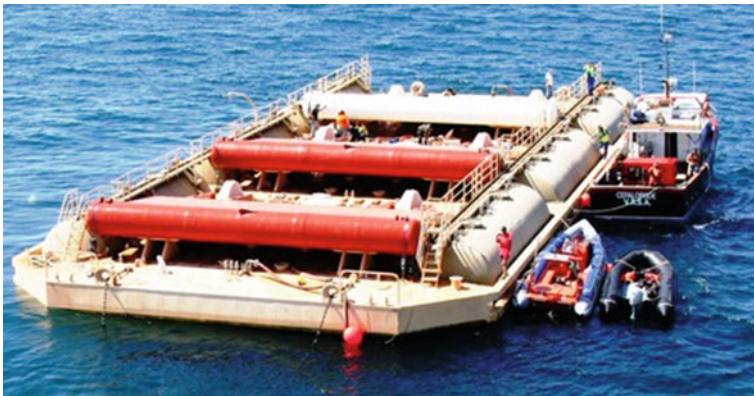
Fig. 18 Waveroller WEC prototype, before submerged to seabed [35]
