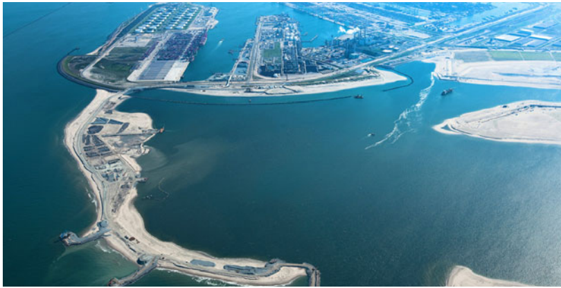
Fig. 8.41 b Artificial beach nourishment at the Tweede Maasvlakte, Rotterdam in The Netherlands (Photo credit: ©Van Oord)
