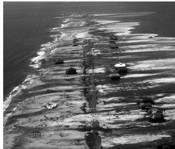
Fig. 8.4b Dramatic shoreline erosion and large overwash deposits along Dauphin Island during Hurricane Katrina (2005) demonstrate classic barrier island rollover. (Photo credit: USGS)
