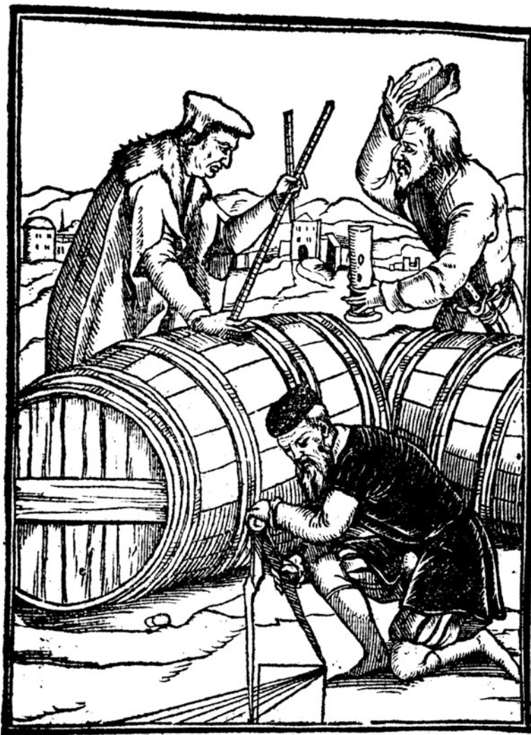
Fig. 6.1 Wine gauger at work. The man at the front of the picture is constructing a quadratic gauging rod (Mennher 1565, MPM A 3589)
