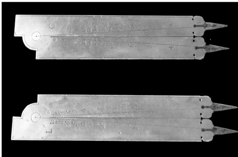
Fig. 7.14 A sector with a scale of inverses on one side and a scale of the sides of an inscribed polygon on the other (private collection)
